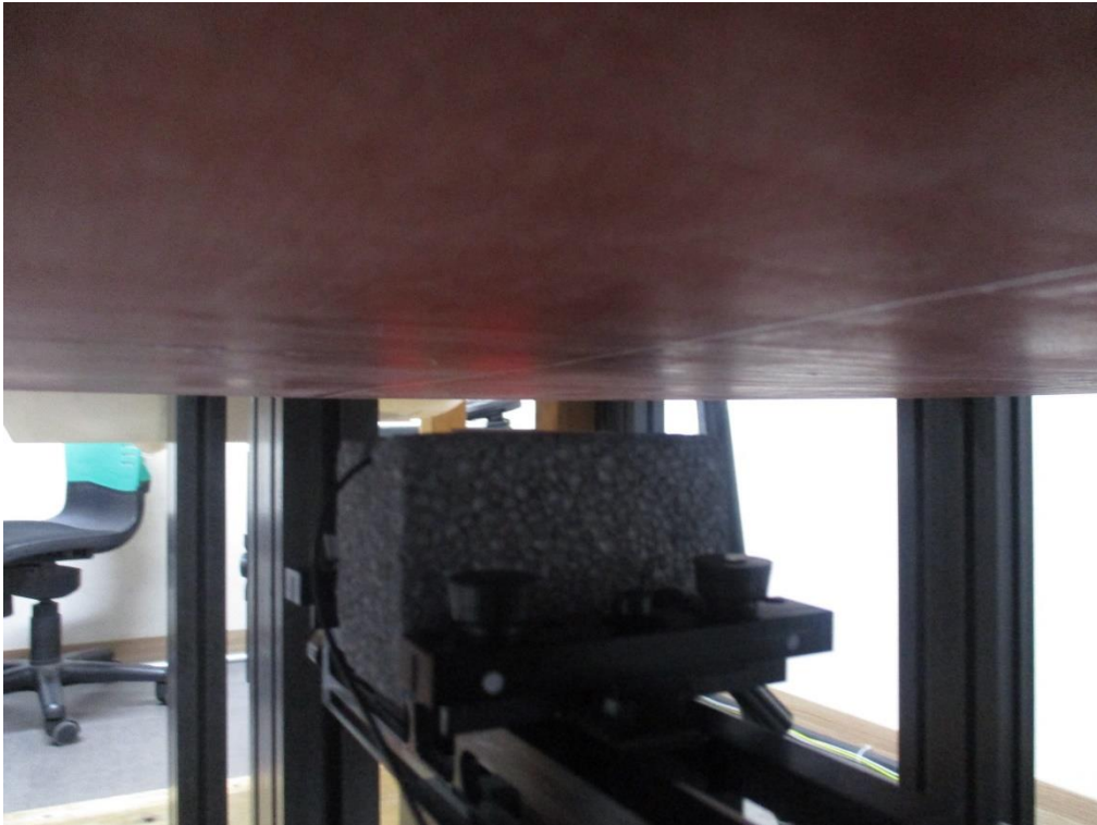
Front Side from Flat Phantom (Separation Distance: 1.5 cm) – Bluetooth Antenna
