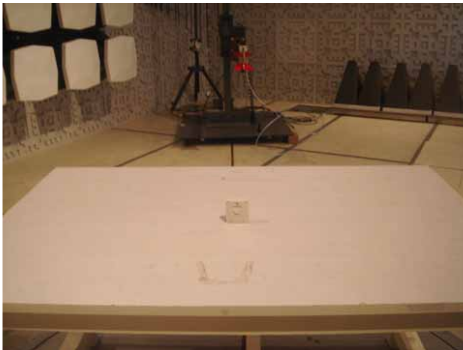
Radiation Emission Test View For 1GHz-5GHz
