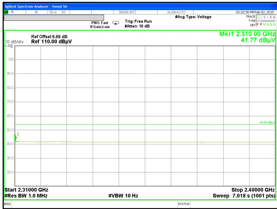
**RESTRICTED BANDEDGE (HIGH CHANNEL, HORIZONTAL) – ECG ½ WAVE DIPOLE**
