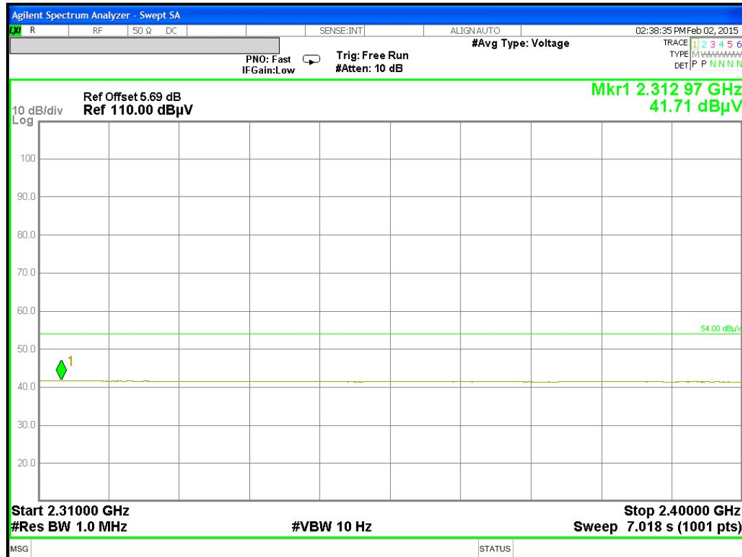
**RESTRICTED BANDEDGE (HIGH CHANNEL, HORIZONTAL) – ECG ¼ WAVE MONOPOLE**
