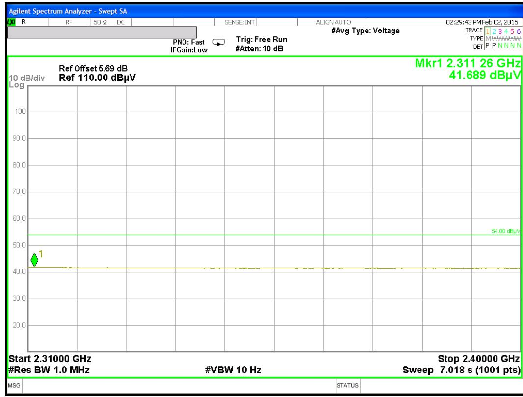
**RESTRICTED BANDEDGE (LOW CHANNEL, VERTICAL) – ECG ½ WAVE DIPOLE**
