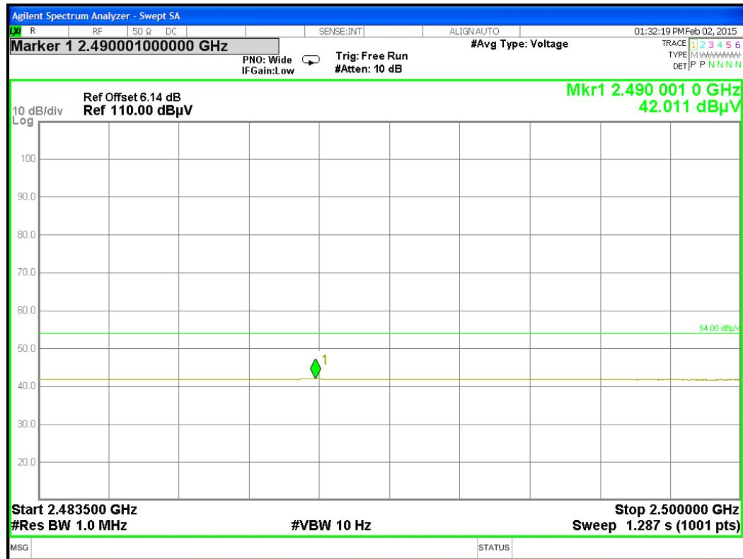
**RESTRICTED BANDEDGE (HIGH CHANNEL, VERTICAL) – ECG 1/4 WAVE MONOPOLE**
