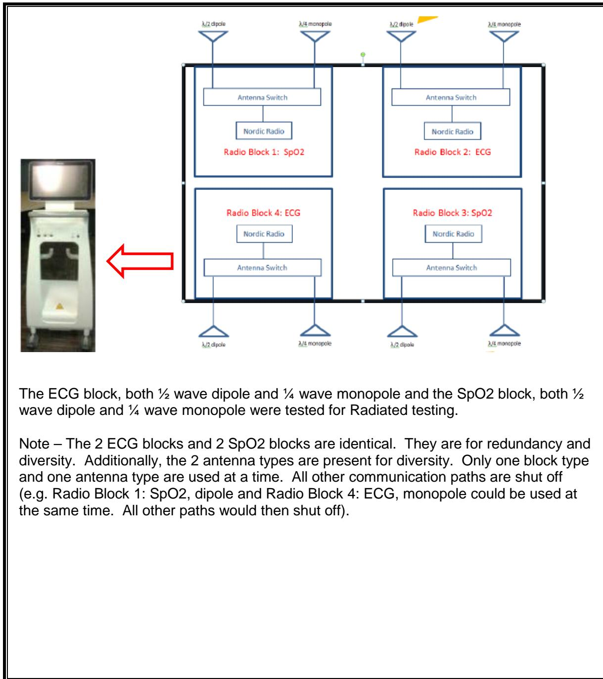
The ECG block, both  $\frac{1}{2}$  wave dipole and  $\frac{1}{4}$  wave monopole and the SpO2 block, both  $\frac{1}{2}$  wave dipole and  $\frac{1}{4}$  wave monopole were tested for Radiated testing.
