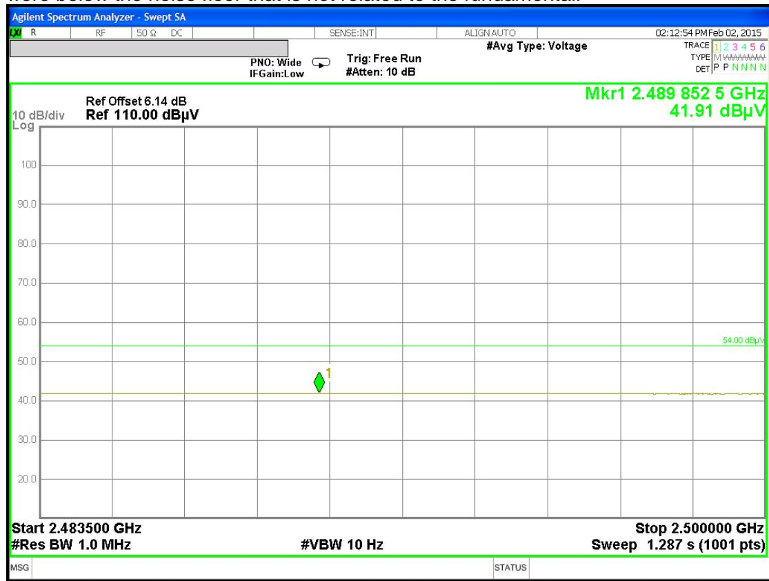
**RESTRICTED BANDEDGE (HIGH CHANNEL, VERTICAL) – ECG ½ WAVE DIPOLE**
