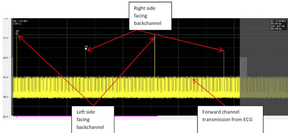
Note – The highest amplitude signal is the transmit signal of the left MR400 ECG Block radio. The lower amplitude signal is the transmit signal of the right MR400 ECG Block with attenuation (for this measurement to differentiate the two signals). The lowest amplitude signal is the received signal from the wECG module (not part of this evaluation and report).
