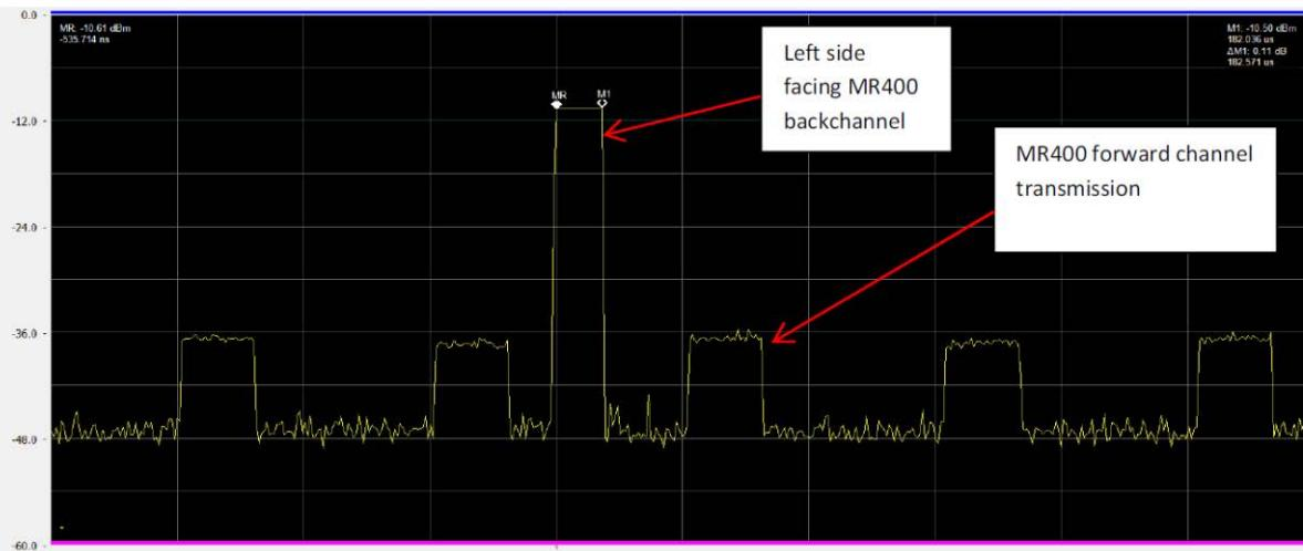
Note - The lower signal channels are the received signals from the wECG. The higher amplitude signal is the MR400 ECG. Invivo states that the SpO2 signals are the same as the ECG signals.
