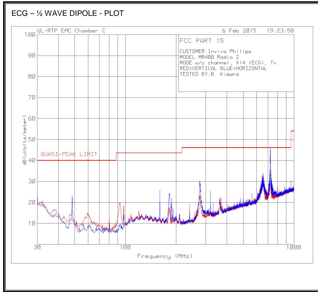
Note – It was determined during testing that the 723 MHz signal was associated with the host (IBP or Invasive Blood Pressure).
