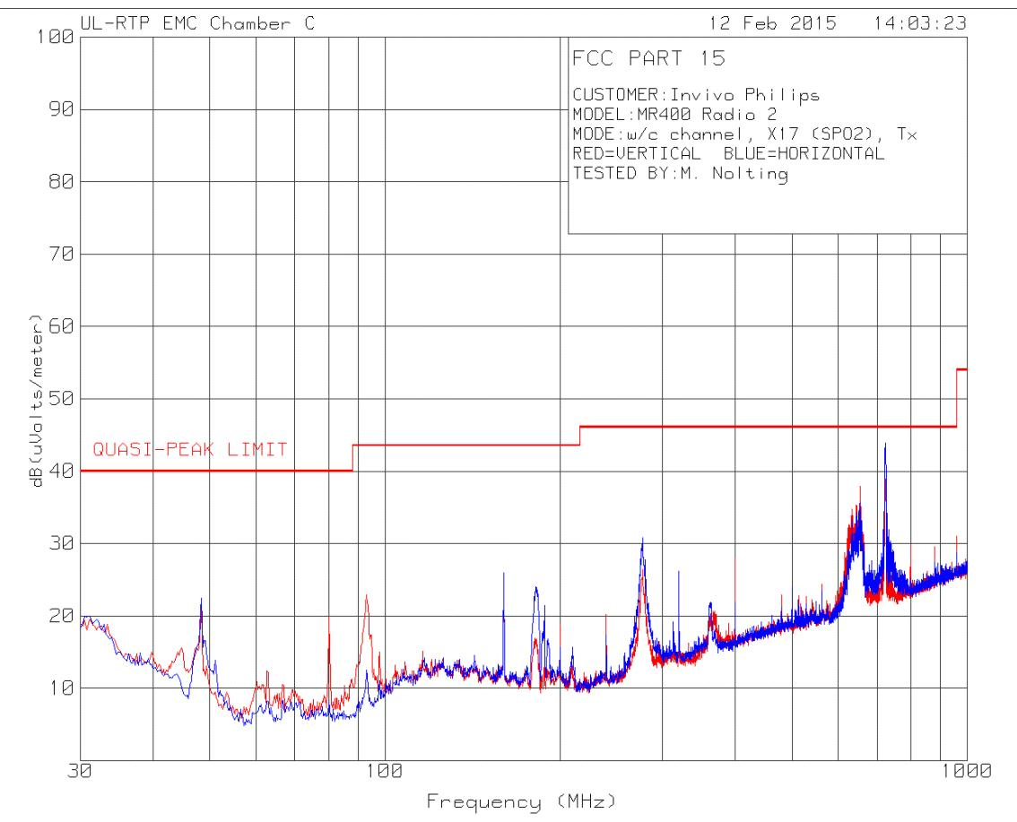
Note – It was determined during testing that the 723 MHz signal was associated with the host (IBP or Invasive Blood Pressure).
