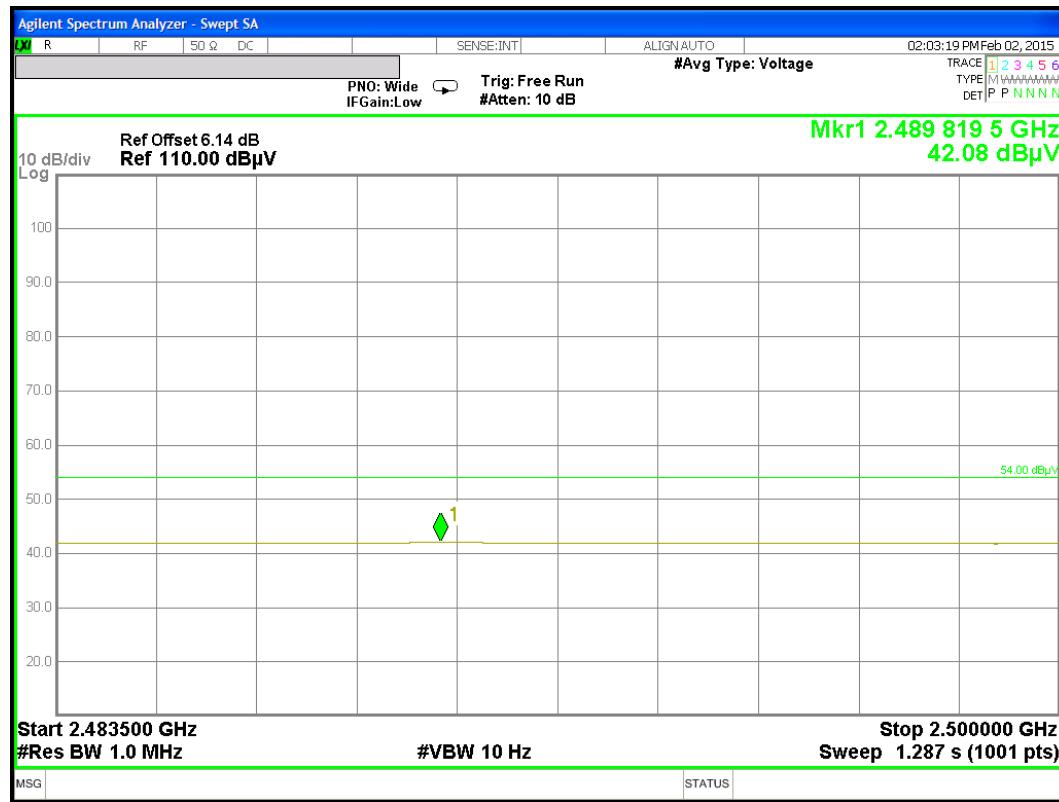
**RESTRICTED BANDEDGE (LOW CHANNEL, HORIZONTAL) – ECG 1/4 WAVE MONOPOLE**
