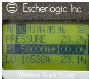
Fig 4.3.5 Sensor Calibration - Setting Loaded Pressure Value
