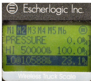
Fig 4.2.5 Sensor Calibration - Setting Empty Weight Value
