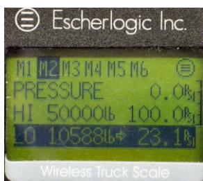
Fig 4.2.6 Sensor Calibration - Setting Empty Pressure Value
