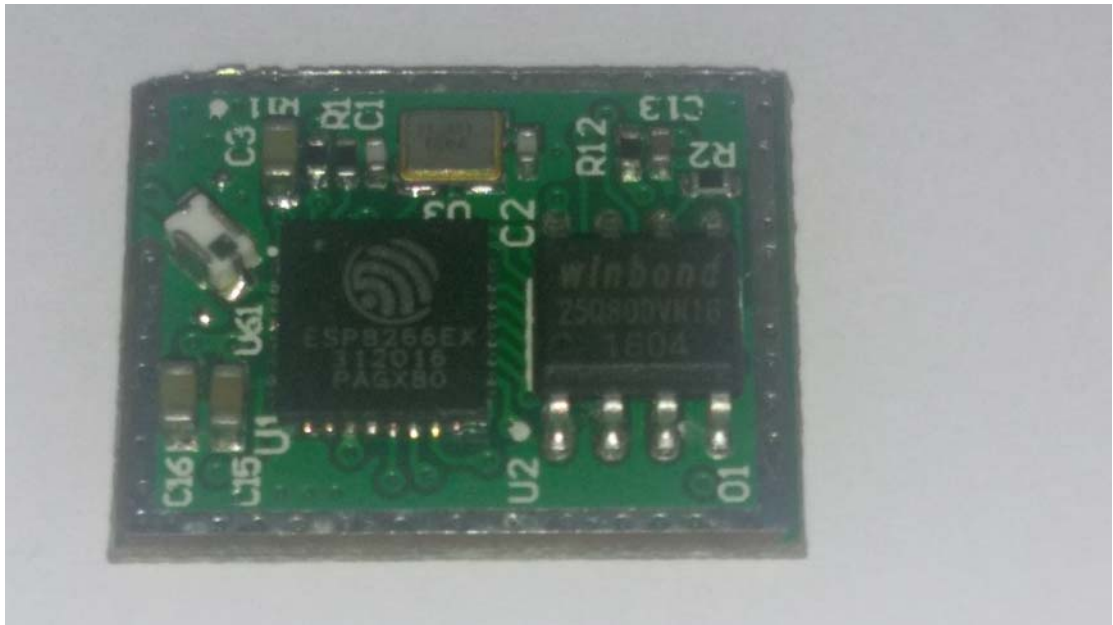
Top with CAN removed
