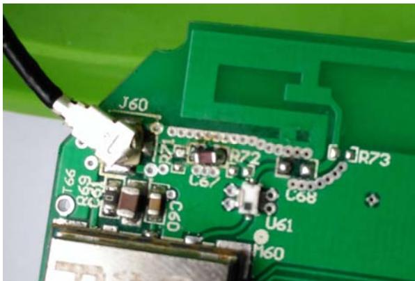
U.FL connector clipped onto PCB.
