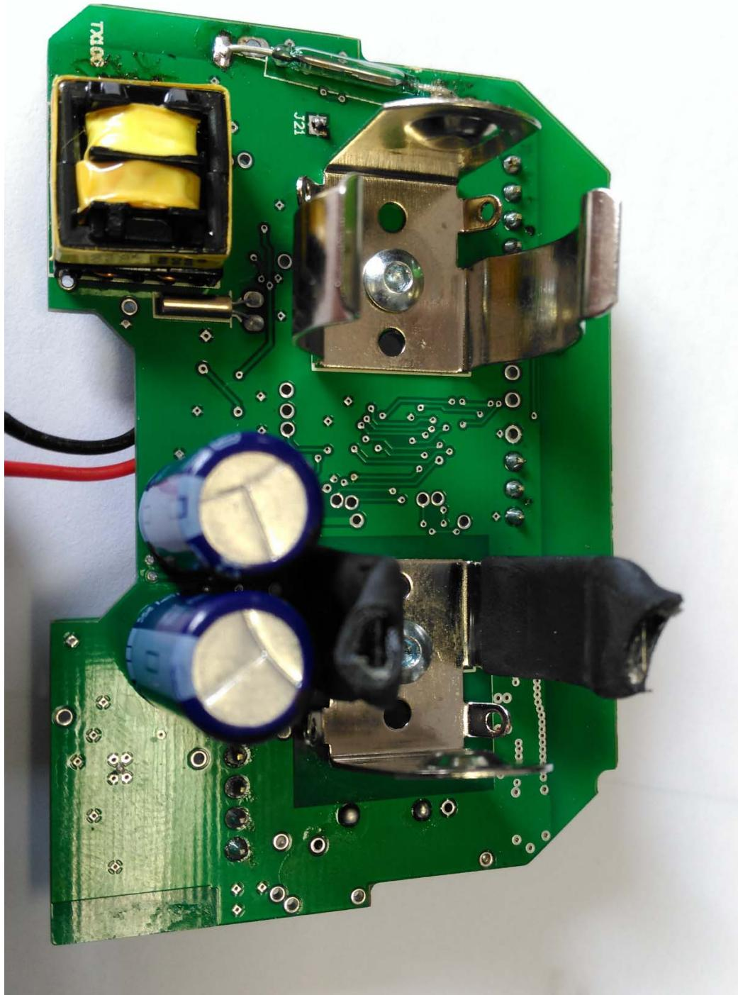
PCB with battery (lithium thioyl chloride) Ultrasonic transducer inserted in horn of enclosure.
