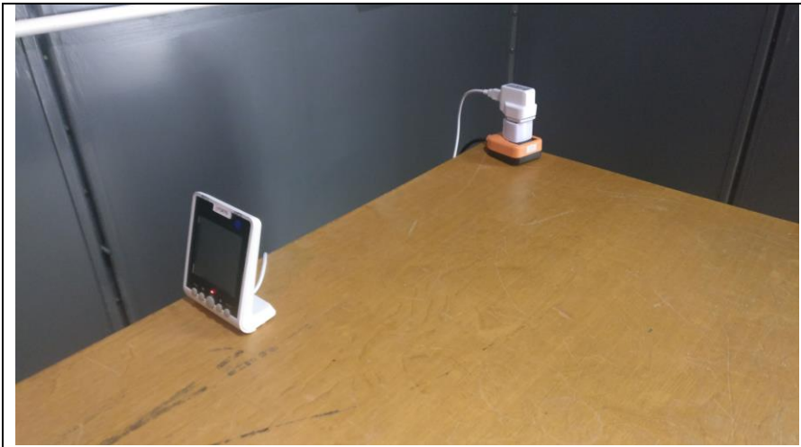
Fig 5a Test setup Conducted Emissions on the mains
