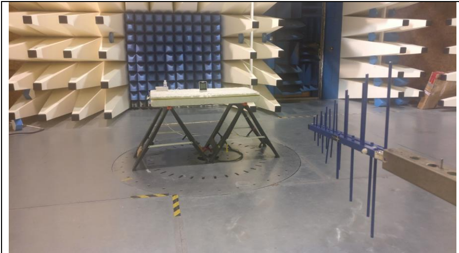
Fig 2a Test setup 300MHz -1GHz Rad Emissions
