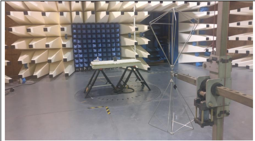
Fig 1a Test setup 30MHz -300MHz Rad Emissions
