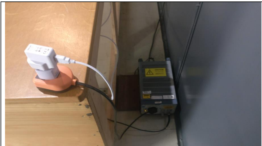
Fig 5b Test setup Conducted Emissions on the mains
