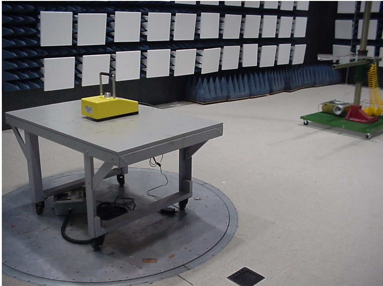
Figure 6 - Radiated Emissions Test Setup (Chamber - Back)
