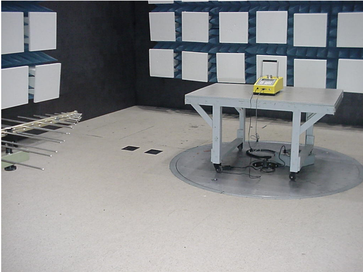
Figure 5 - Radiated Emissions Test Setup (Chamber - Front)
