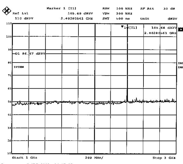
**Out of Band Emission(Antenna Terminal Conducted): FCC 15.247(d)**
