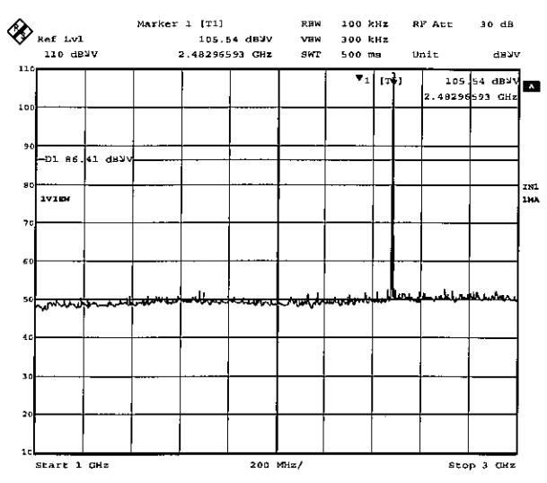
**Out of Band Emission(Antenna Terminal Conducted): FCC 15.247(d)**
