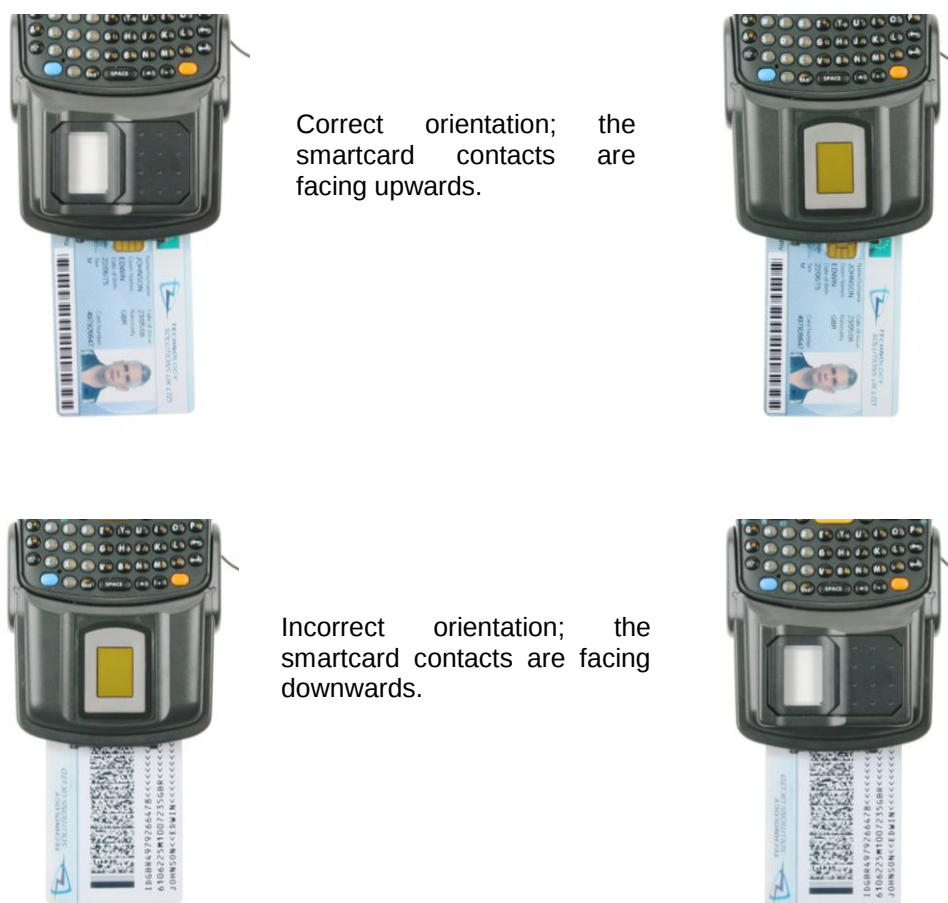
Figure 5: Inserting a smartcard into the Tri-Scan 1084
