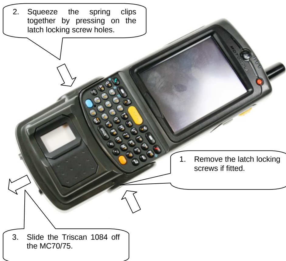
Figure 4: Detaching from an MC70/75
