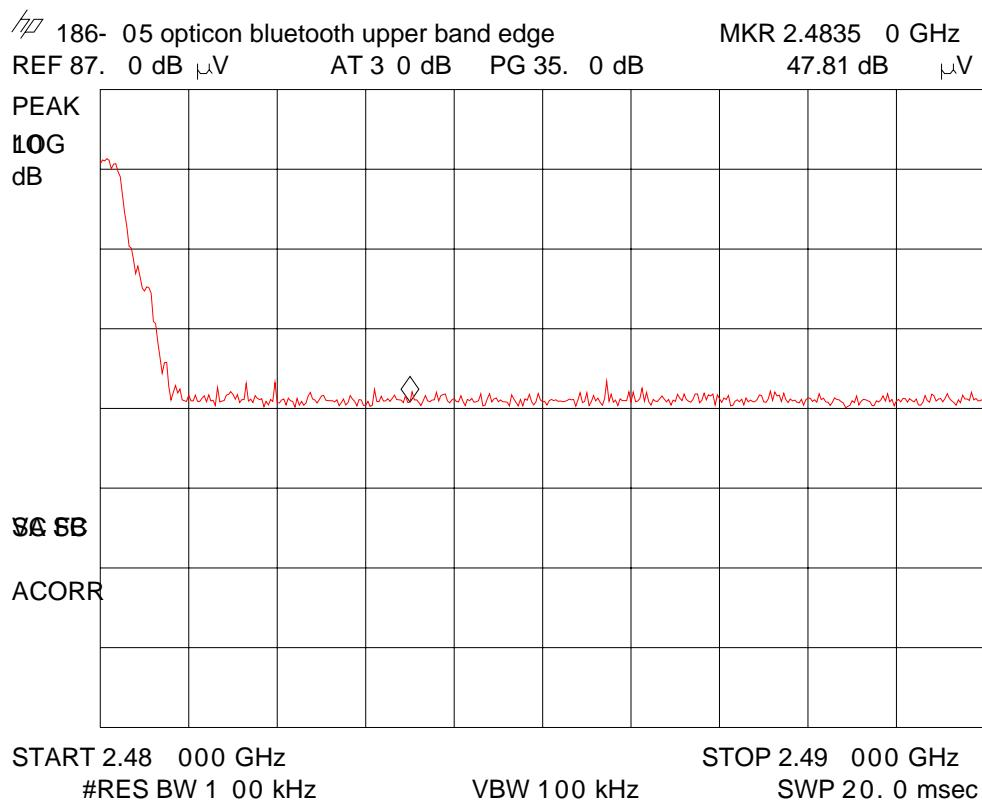
Marker is at the band edge 2483.5MHz, the limit is 54 dBuV/m at 3m, EUT meets this limit by 6.19dB using a peak detector.
