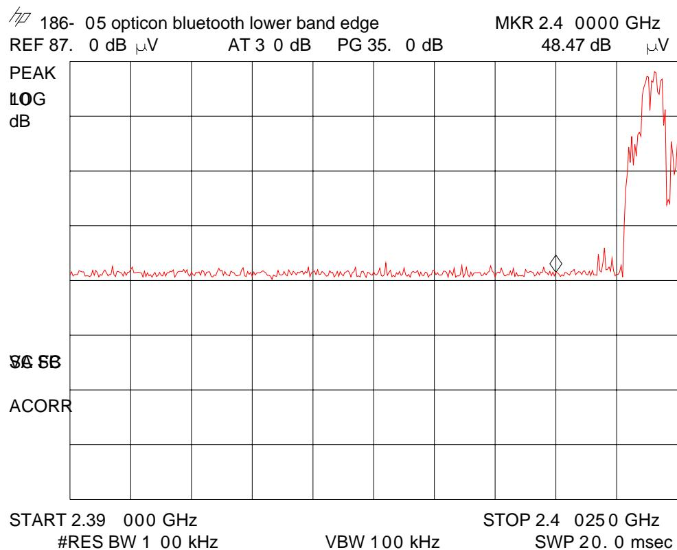
Marker is at the band edge 2400MHz, the limit is 54 dBuV/m at 3m, EUT meets this limit by 5.53dB using a peak detector.
