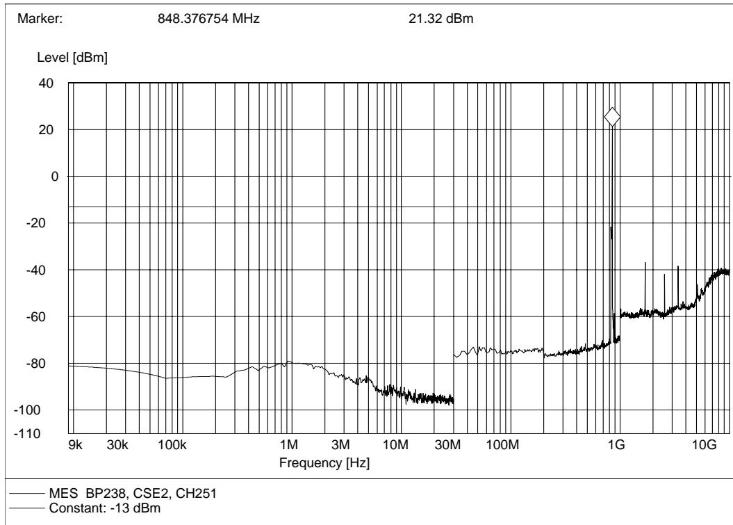
**Plot of Mobile Station Emissions in the base station frequency range**
