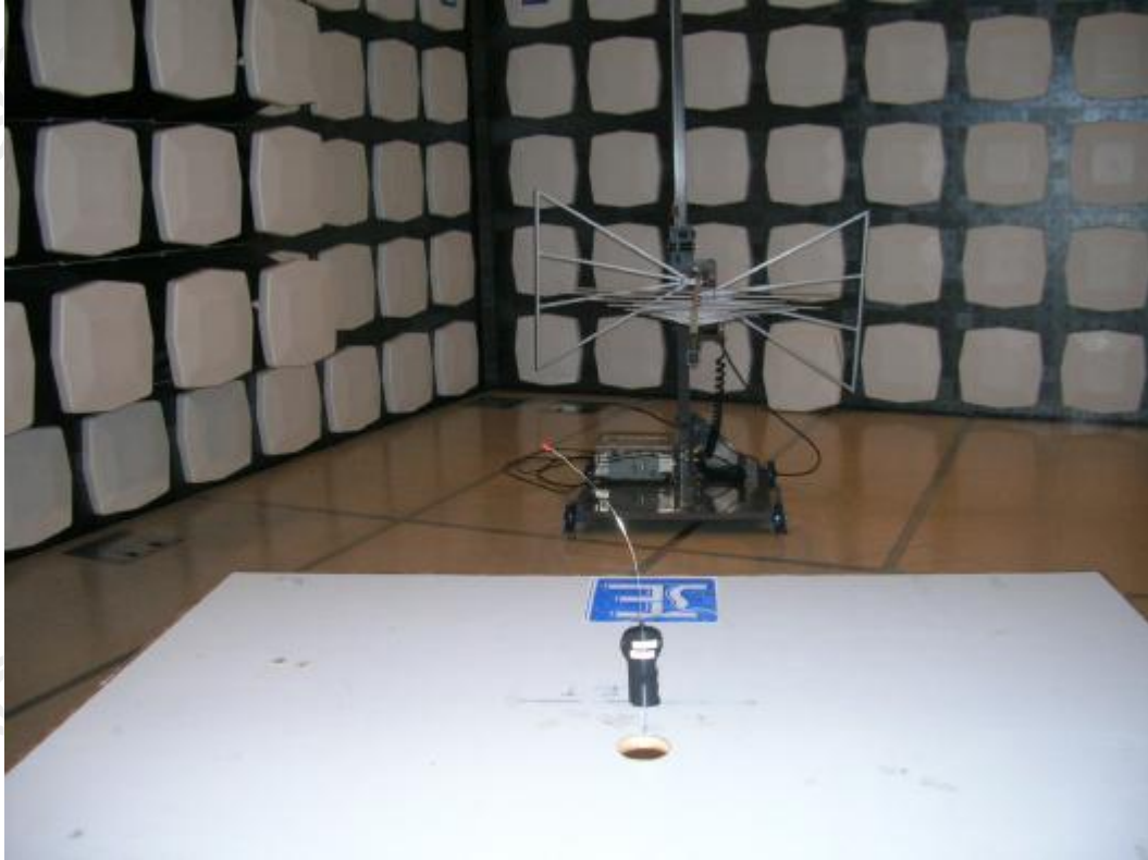
Measurement of Radiated Emission Test Set Up
