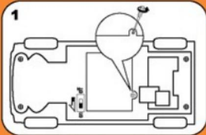
1. Make sure the ON/OFF switch is in the "OFF" position on toy. Remove the screws on the battery lid. Remove lid to access the battery compartment.
