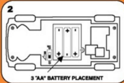
2. Insert 3 "AA" batteries into battery compartment. Close the battery lid, reattach screw to battery lid to lock. Turn the ON/OFF switch to "ON" position.
