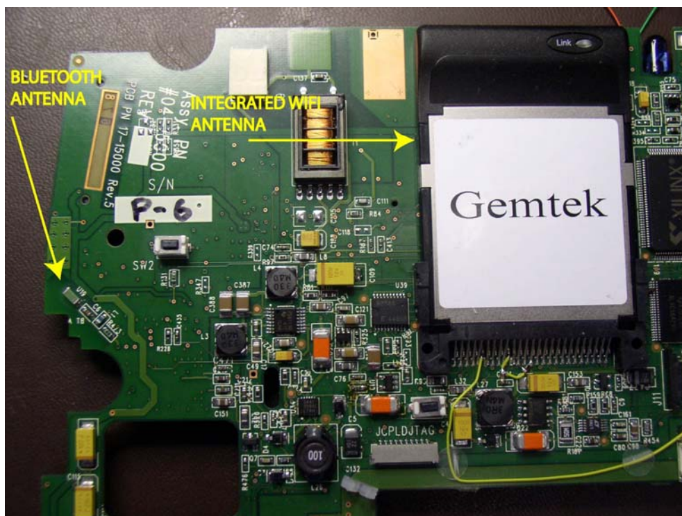
Photograph 4. Location of EUT Antennas
