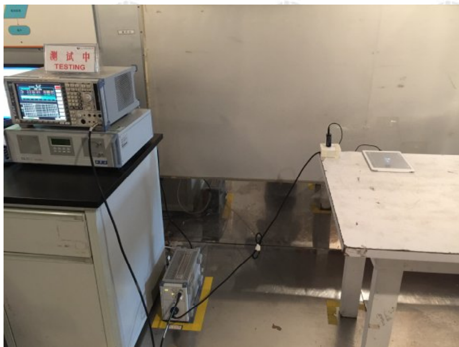
Conducted emission Test Setup
