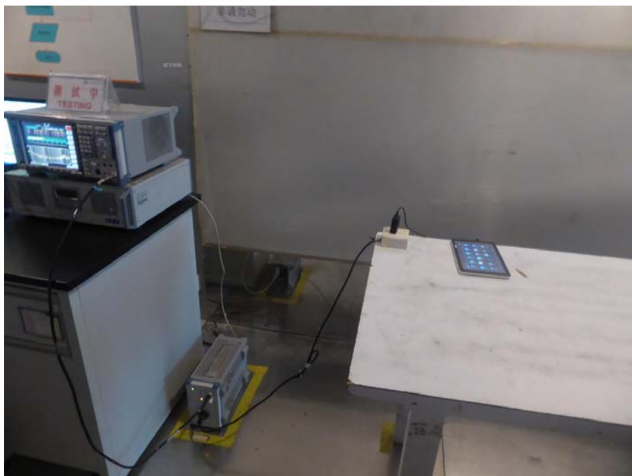
Conducted emission Test Setup
