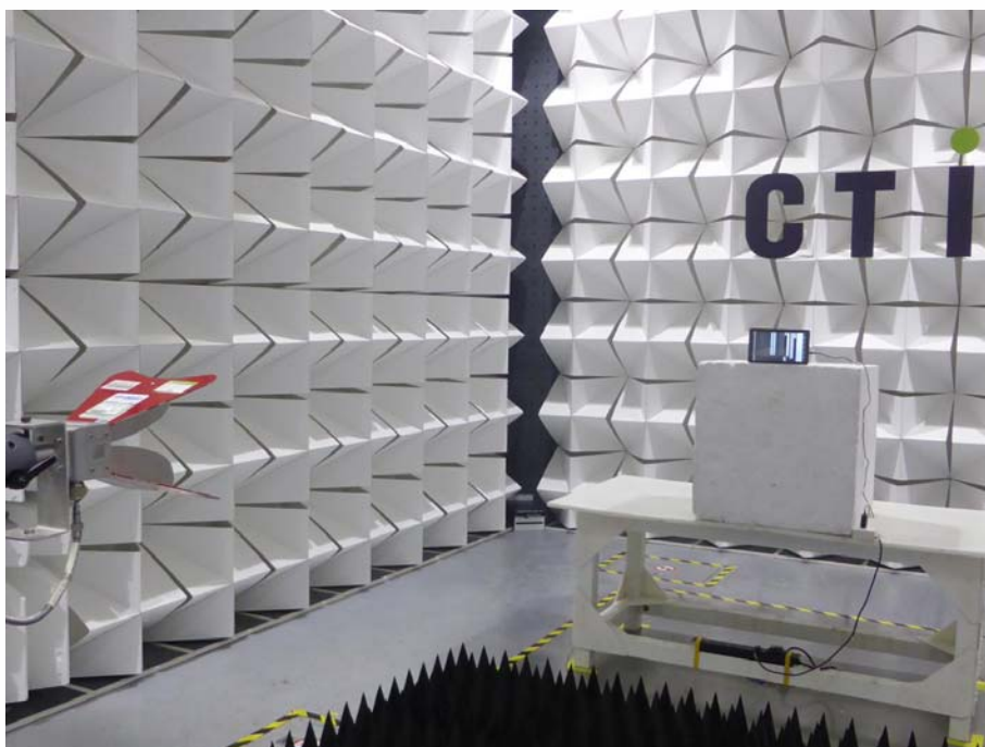
Radiated spurious emission Test Setup-2(Above 1GHz)
