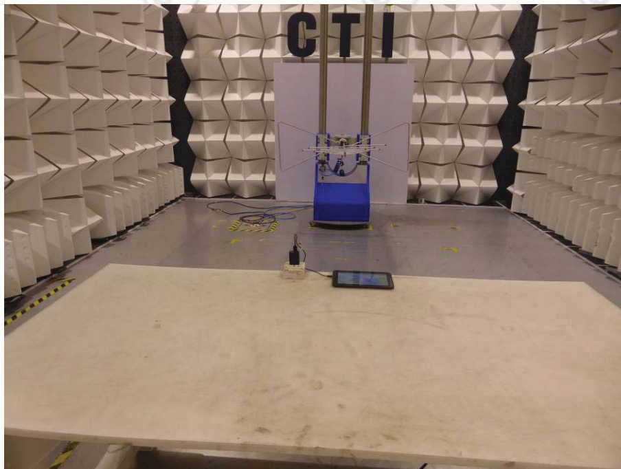
Radiated spurious emission Test Setup-1(Below 1GHz)
