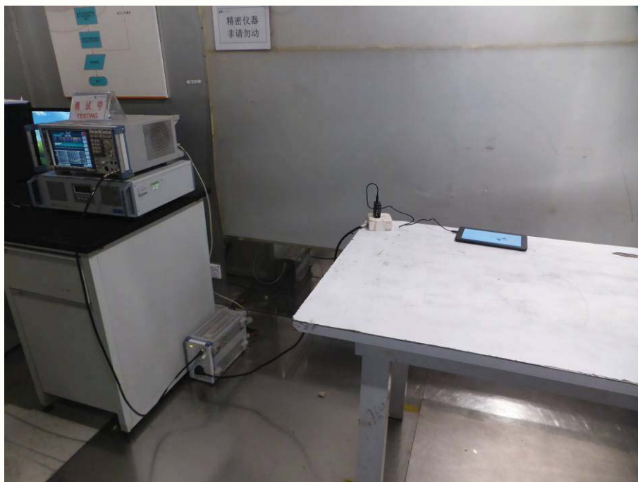
Conducted emission Test Setup
