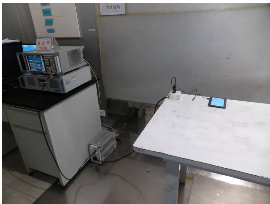
Conducted emission Test Setup
