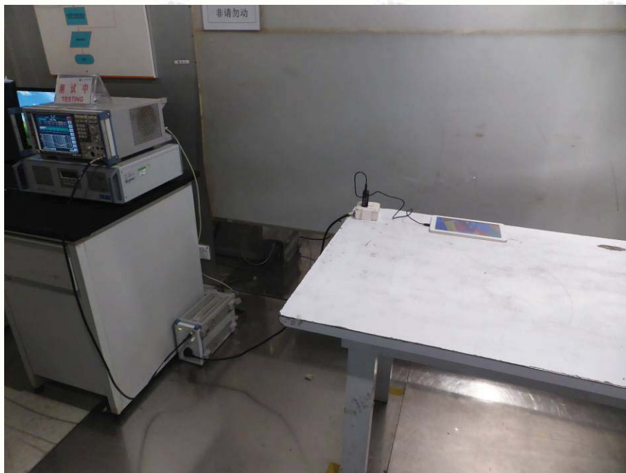
Conducted emission Test Setup
