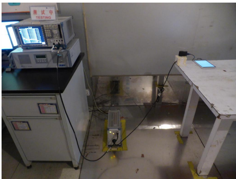
Conducted Emissions Test Setup
