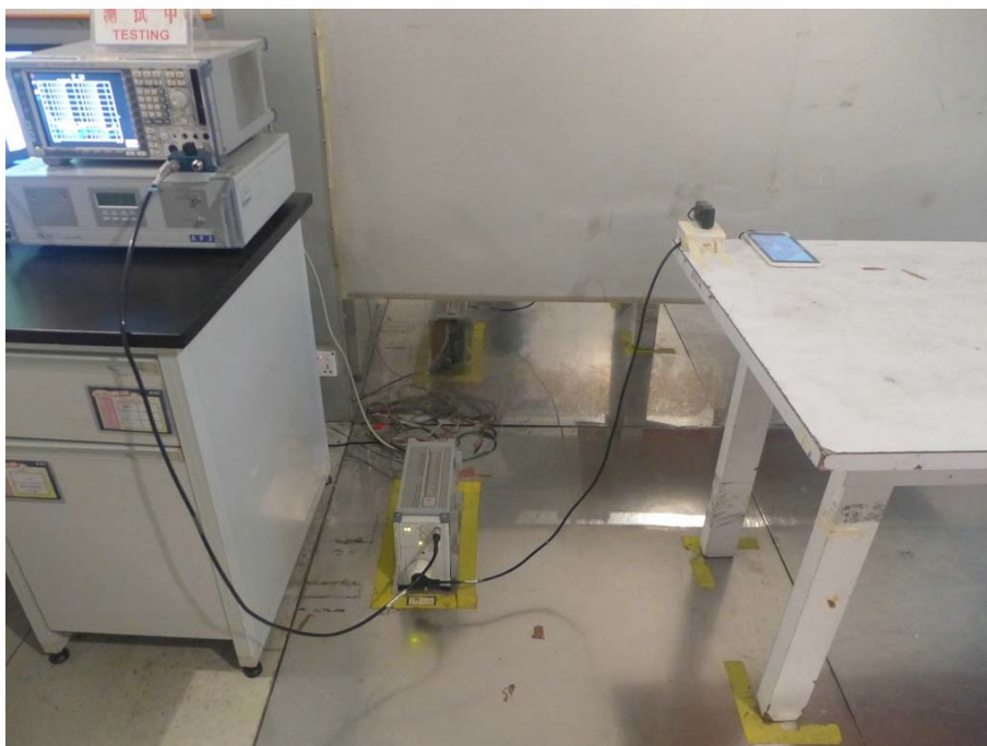
Conducted Emissions Test Setup
