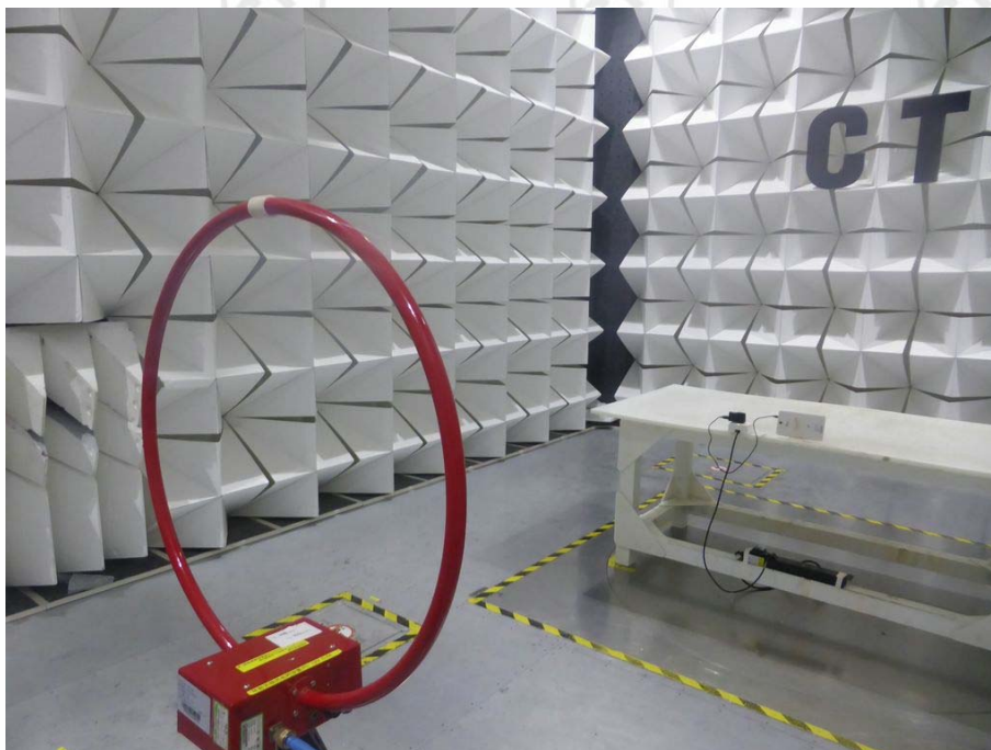
Radiated spurious emission Test Setup-1(Below 30MHz)
