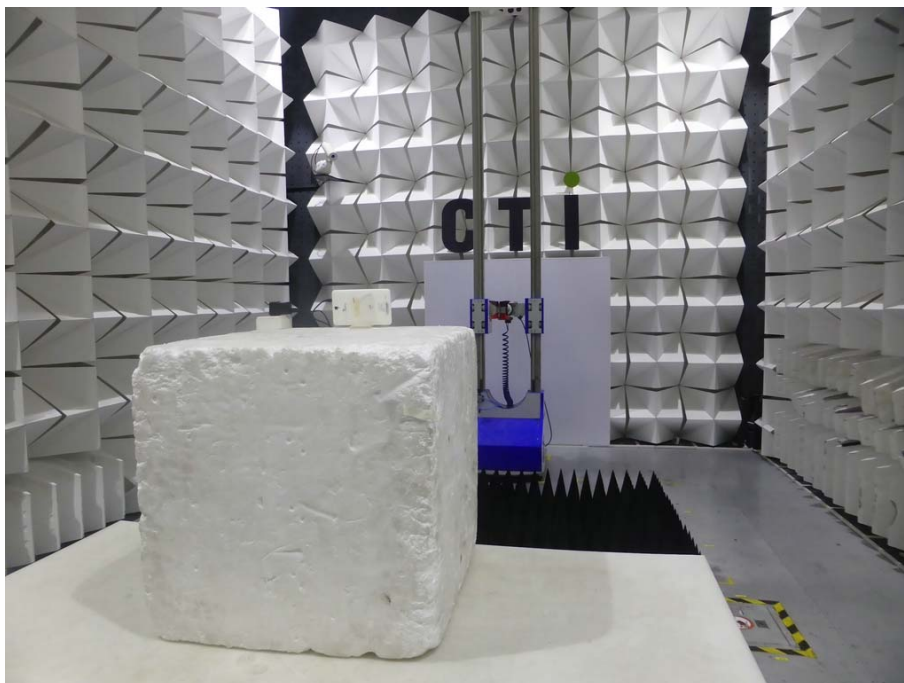
Radiated spurious emission Test Setup-3(Above 1GHz)
