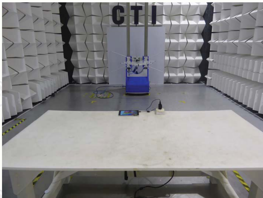
TEST SETUP OF RADIATED EMISSION (30MHz-1GHz)
