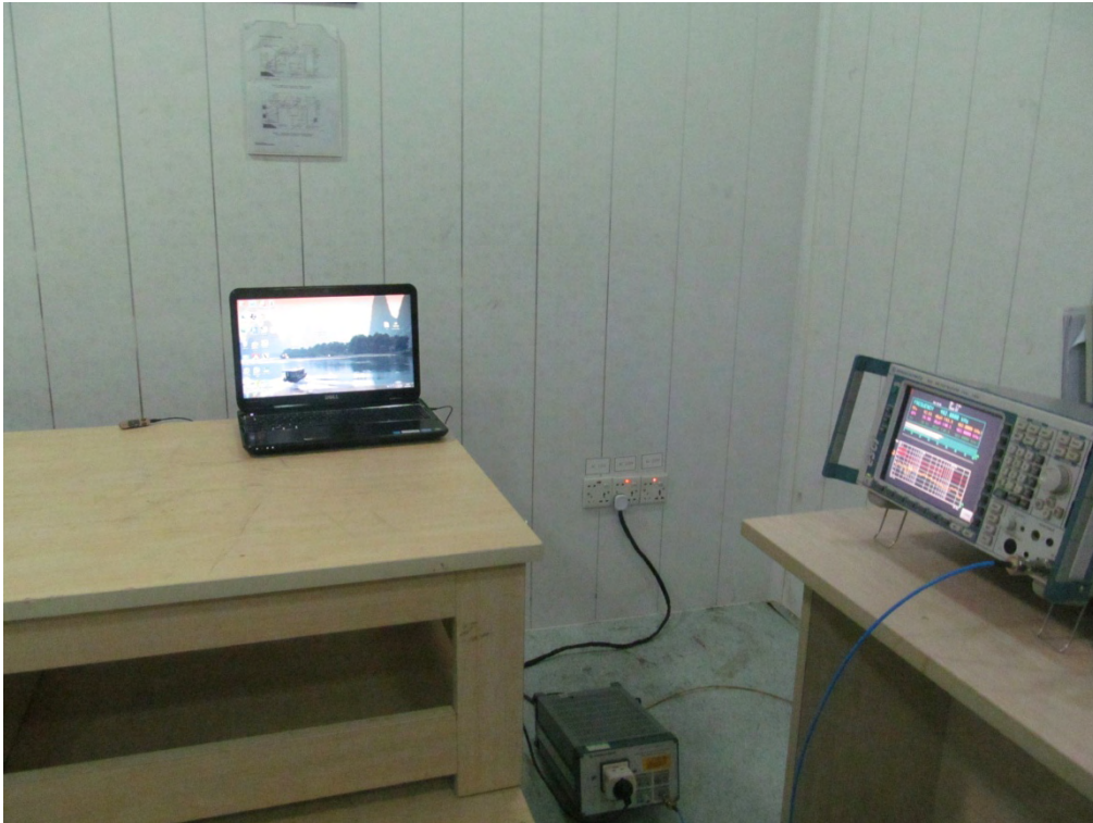
FCC RADIATED EMISSION TEST SETUP
