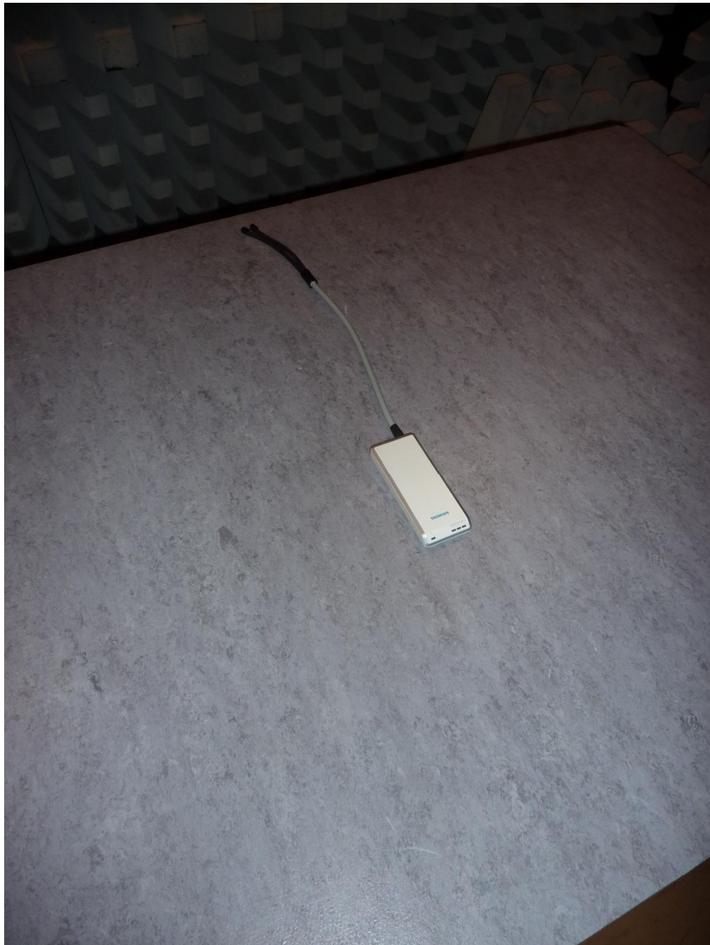
160125_h1.JPG: PPU_098, test setup fully anechoic chamber below 30 MHz (pos. 1)
