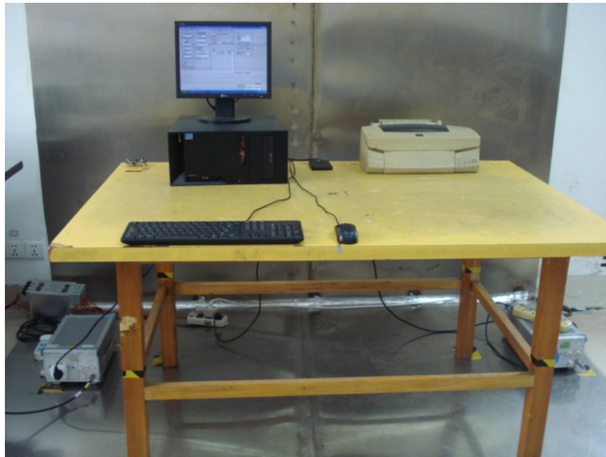
Conducted Emissions Test Setup – Front View
