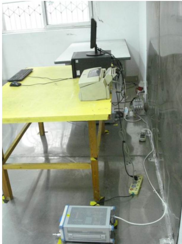
Conducted Emissions Test Setup – Side View
