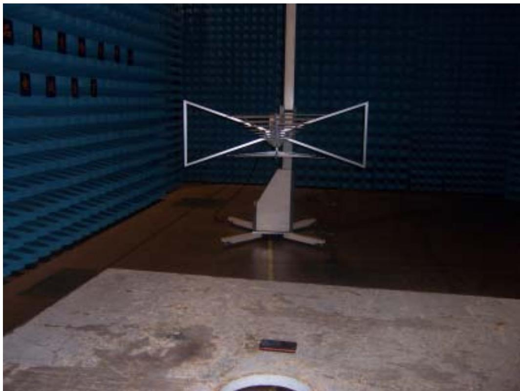
**4. Radiated Emission Test (above 1 GHz)**
