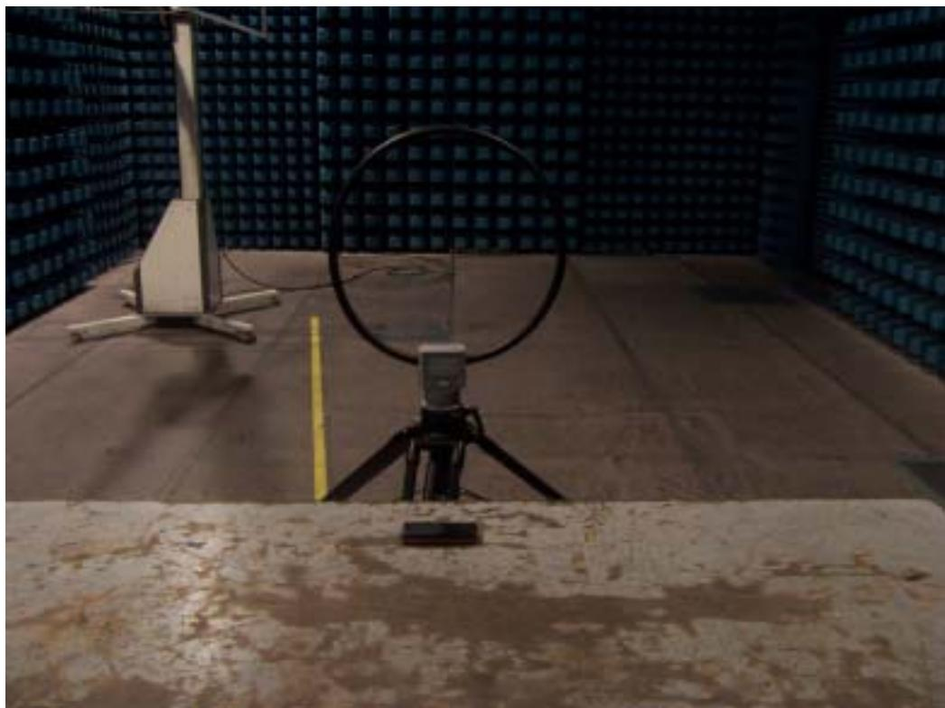
**3. Radiated Emission Test (30 MHz – 1 GHz)**
