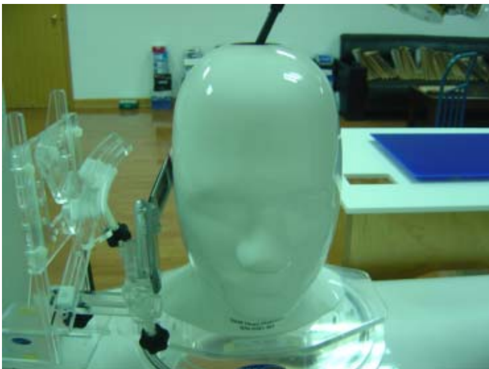
Fig.6 EUT Right Head Tilt15 Position
