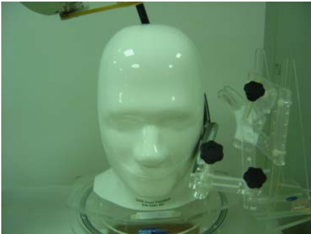
Fig.3 EUT Left Head Touch Cheek Position
