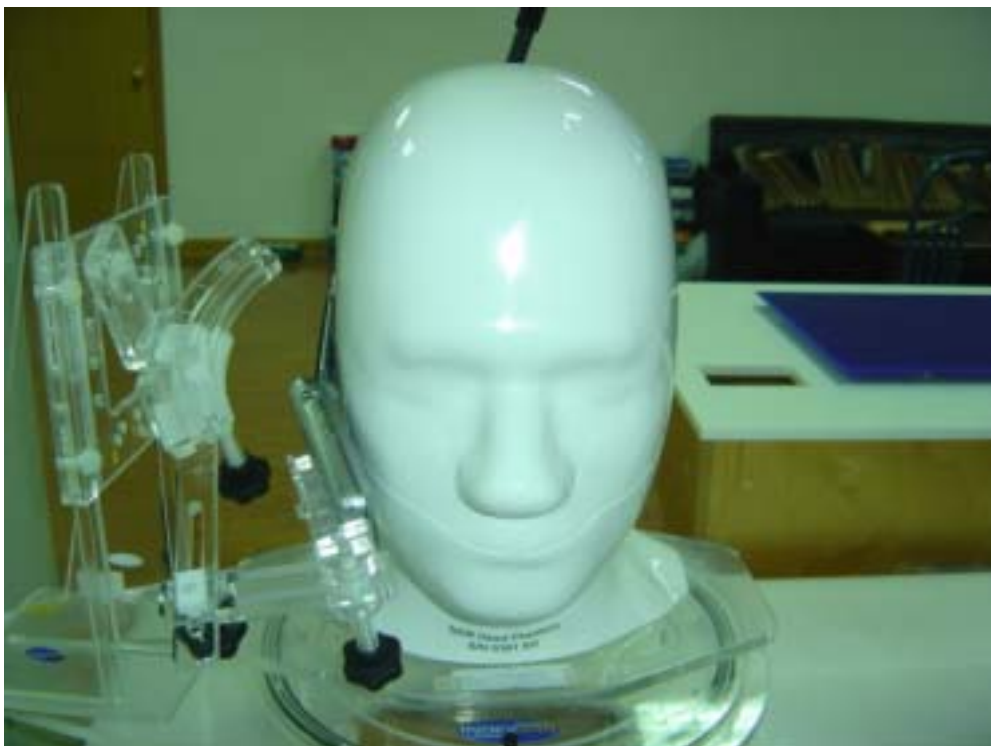
Fig.5 EUT Right Head Touch Cheek Position
