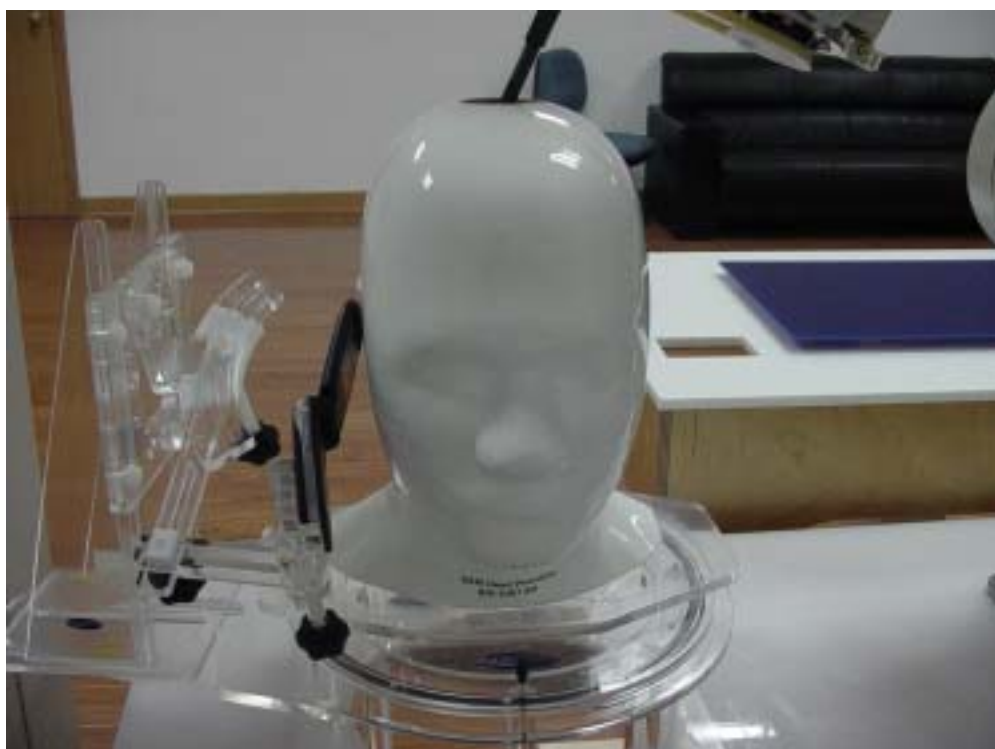
Fig.6 EUT Right Head Tilt15 Position
