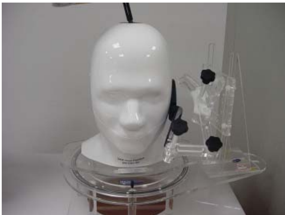
Fig.3 EUT Left Head Touch Cheek Position
