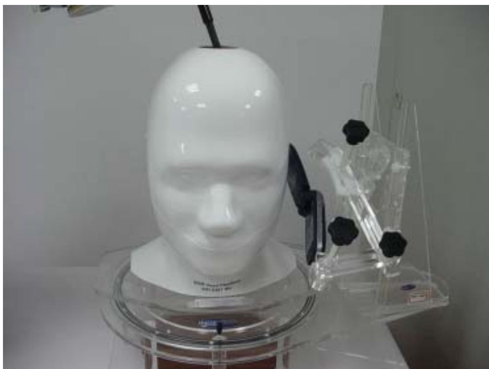
Fig.4 EUT Left Head Tilt15 Position
