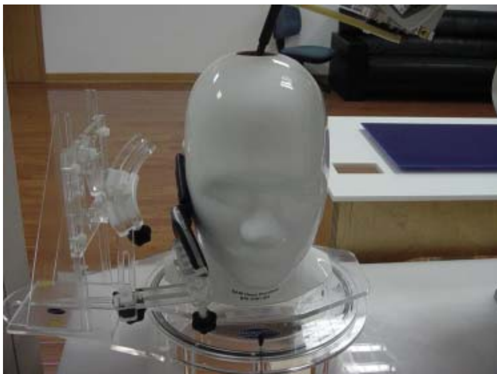
Fig.5 EUT Right Head Touch Cheek Position
