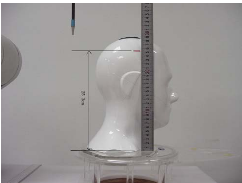
Fig.2 The depth of head tissue in SAM
