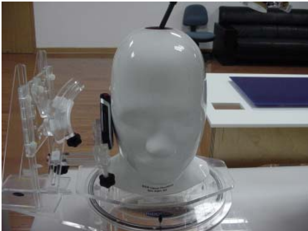
Fig.5 EUT Right Head Touch Cheek Position
