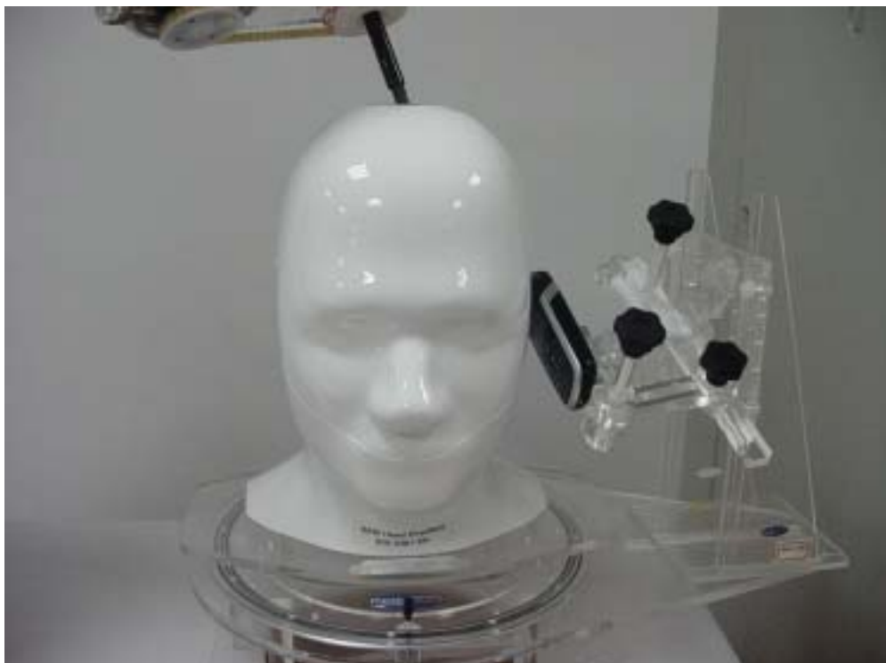
Fig.4 EUT Left Head Tilt15 Position
