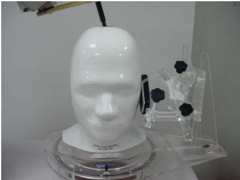
Fig.3 EUT Left Head Touch Cheek Position
