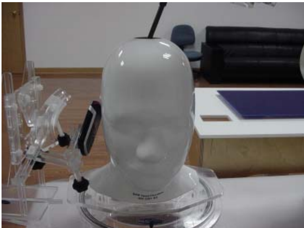
Fig.6 EUT Right Head Tilt15 Position
