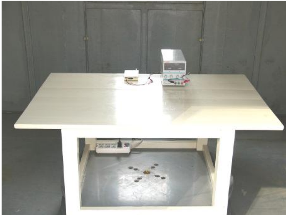
Radiated emission test view – EUT with TLB-915-2.5J Antenna
