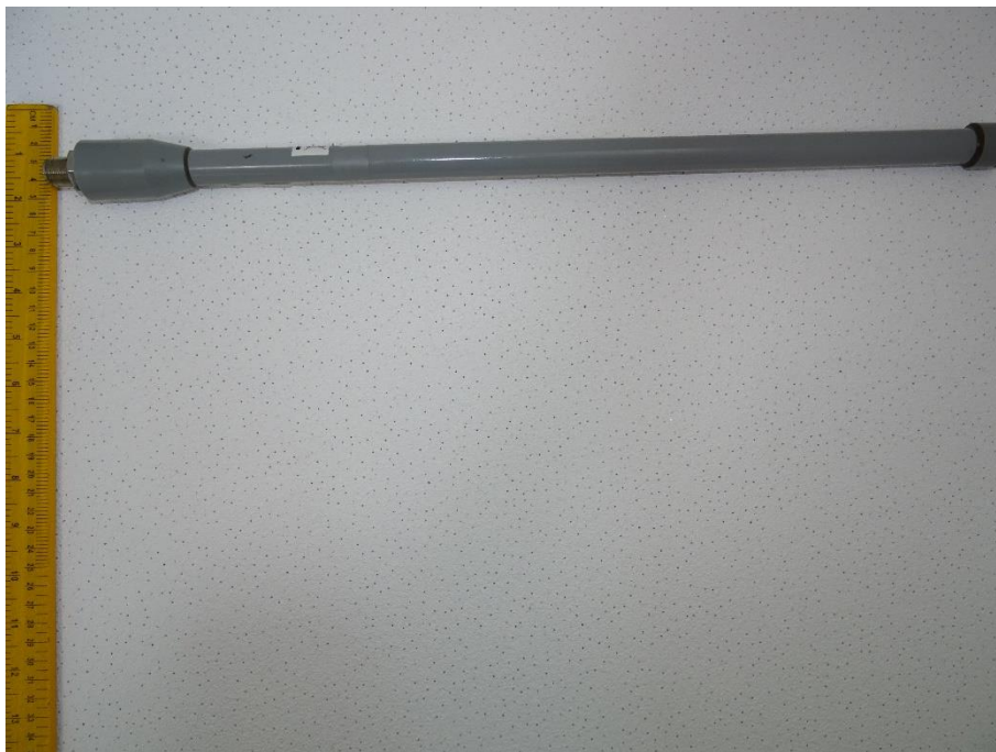
Antenna 4: HGV – 2409 U Omni antenna ( 8 dBi)
