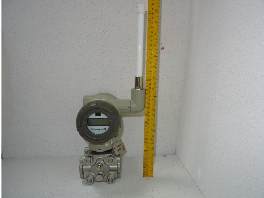
Photo 9: Dimensional view of Host with 4 dBi antenna
