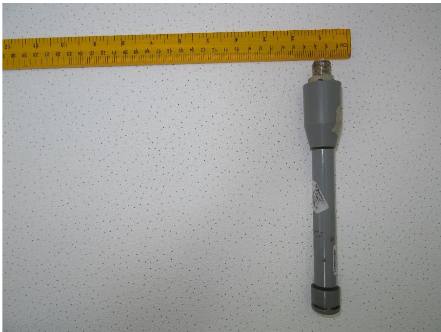
Antenna 3: HGV- 2404U antenna (4 dBi)
