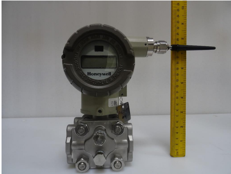
Photo 11: Host with +2 dBi antenna (front view)
