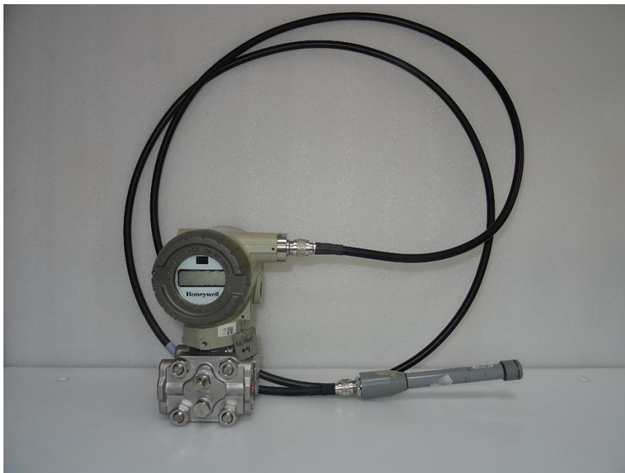
Photo 14: Host with +4 dBi (HGV – 2404U) antenna
