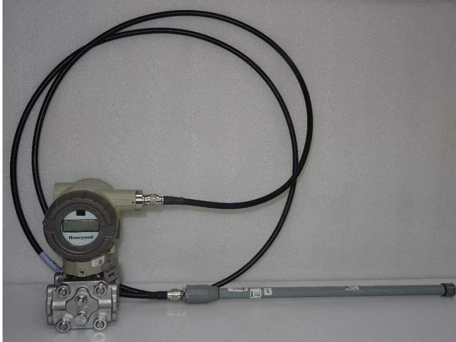
Photo 13: Host with +8 dBi antenna
