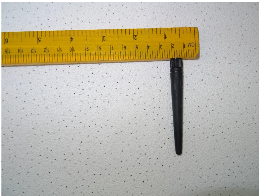
Antenna 1: HG2402RDR-RSP / Rubber Duck Omni antenna (2 dBi)
