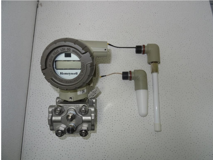
Photo 1: Host device with -2 dBi and 4 dBi antenna
