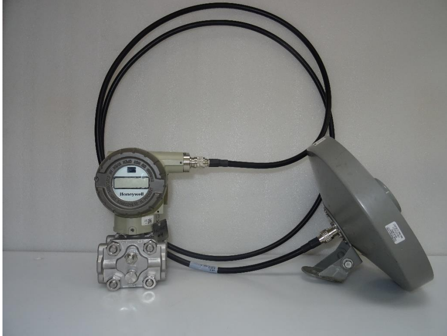
Photo 15: Host with 14 dBi antenna
