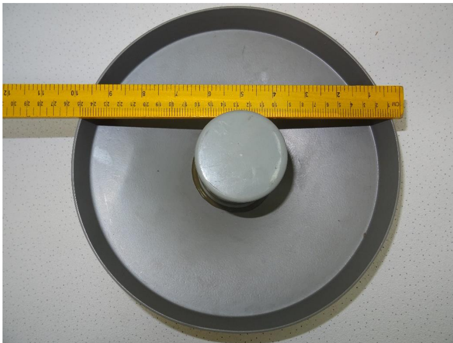
Antenna 5: HG – 2414 D / Dish Antenna (14 dBi)
