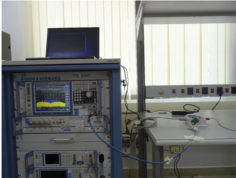
Photo 16: RF module conducted setup - FSV7 analyzer
