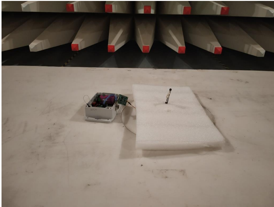
Photo 7: RF module on turn table for below 1000 MHz
