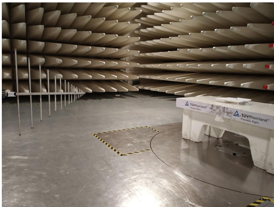
Photo 5: Log periodic antenna - Vertical polarization
