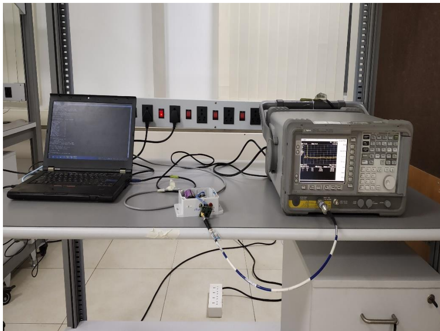
Photo 17: RF module conducted setup - Agilent spectrum analyzer
