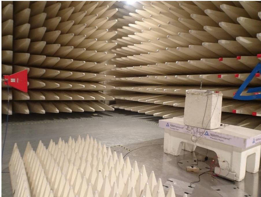
Photo 9: Horn antenna - Horizontal polarization
