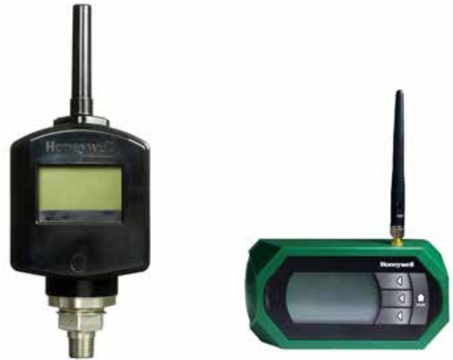
Figure 56. Highest RF signal when antennas are as parallel to each other as possible (parallel arrangement shown Limitless™ WMPR monitor and WPS sensor)
