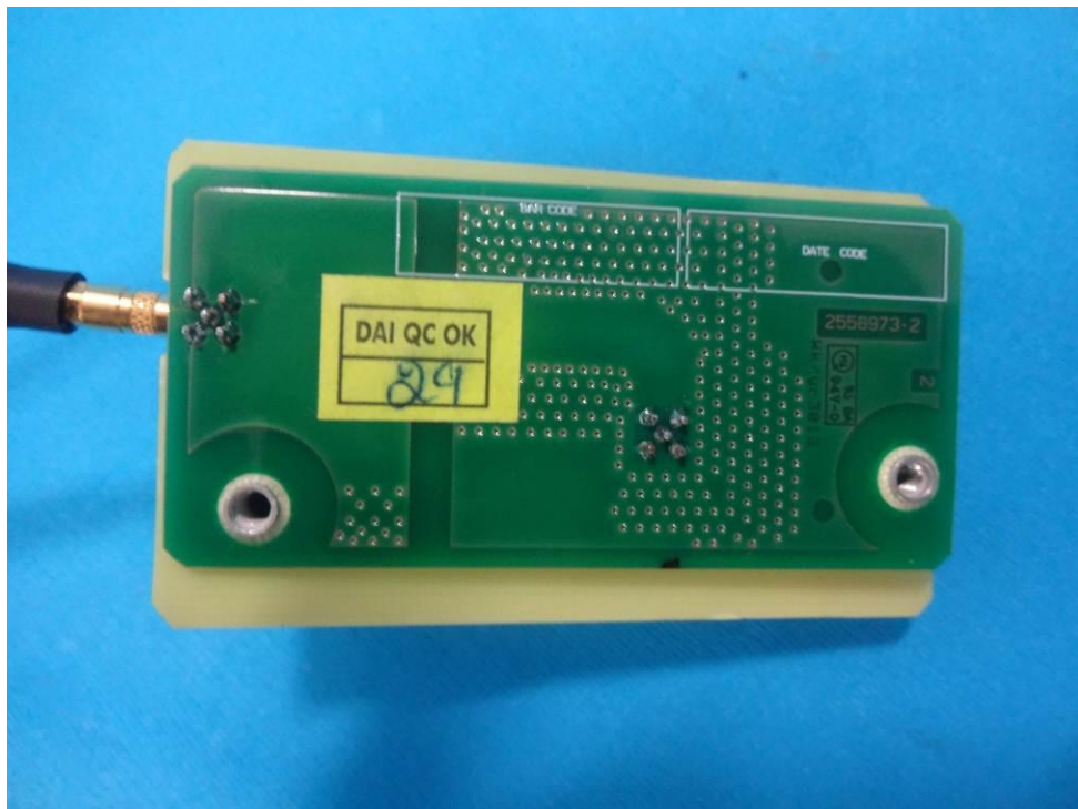
Antenna Connection Board
