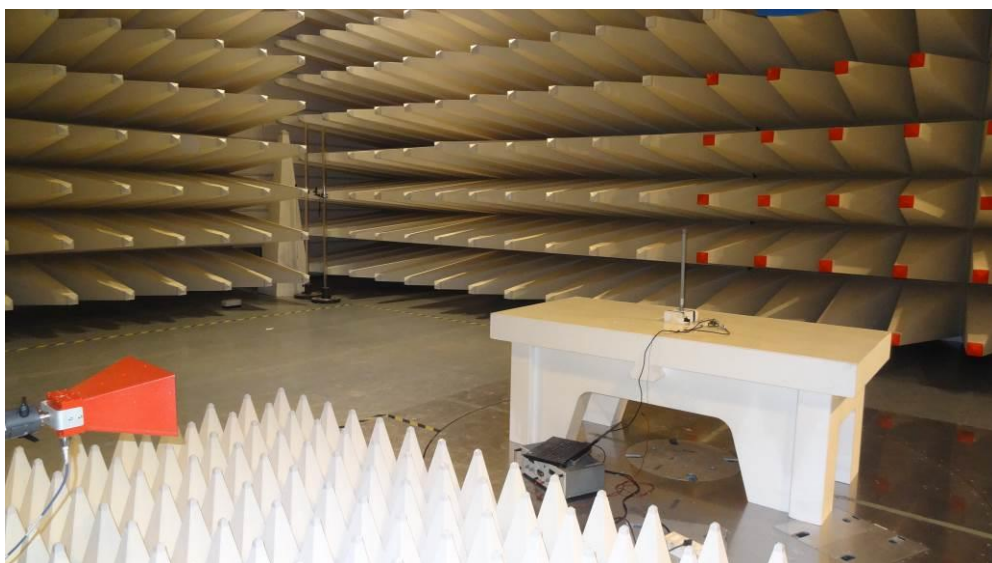
Radiated Test setup
