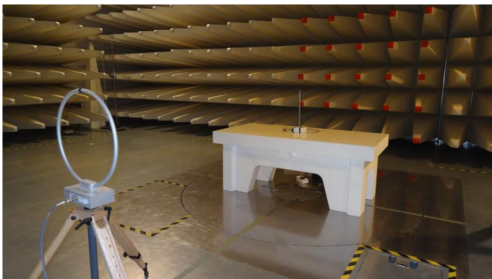
Radiated Test setup
