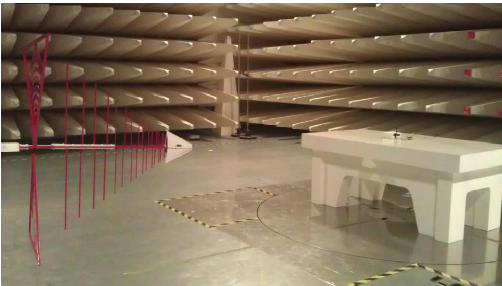
Radiated Test setup
