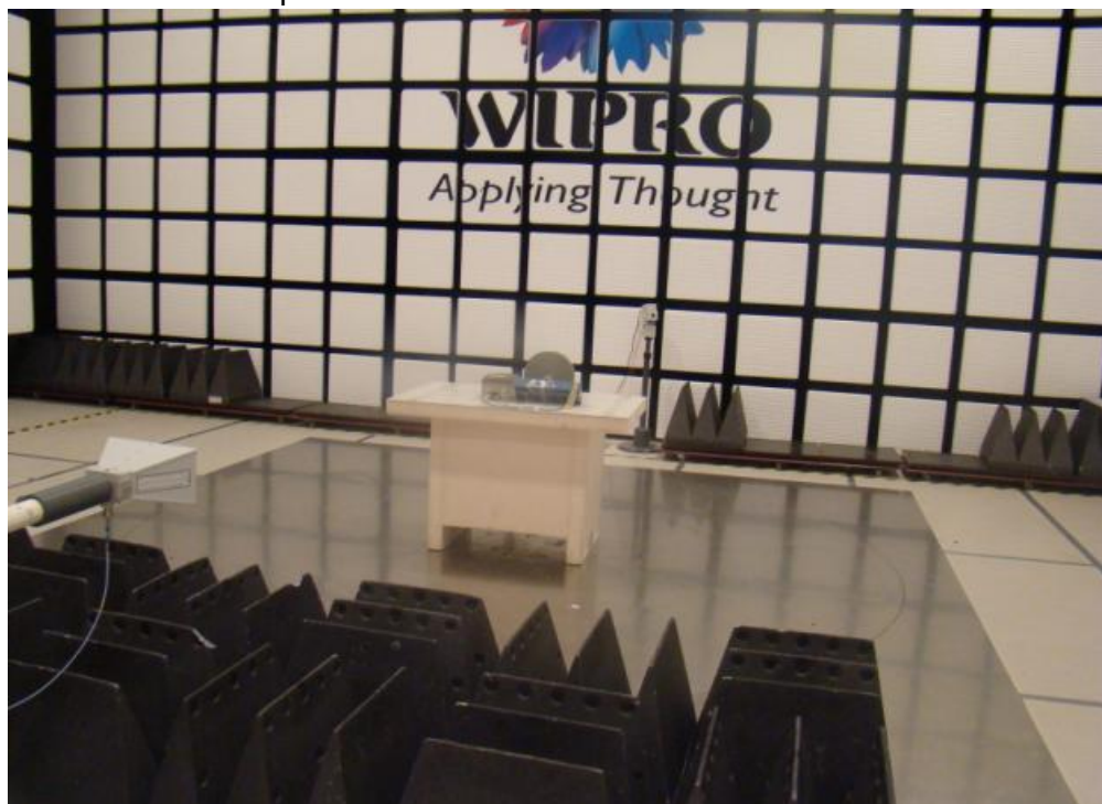
Radiated Test setup: Module inside host
