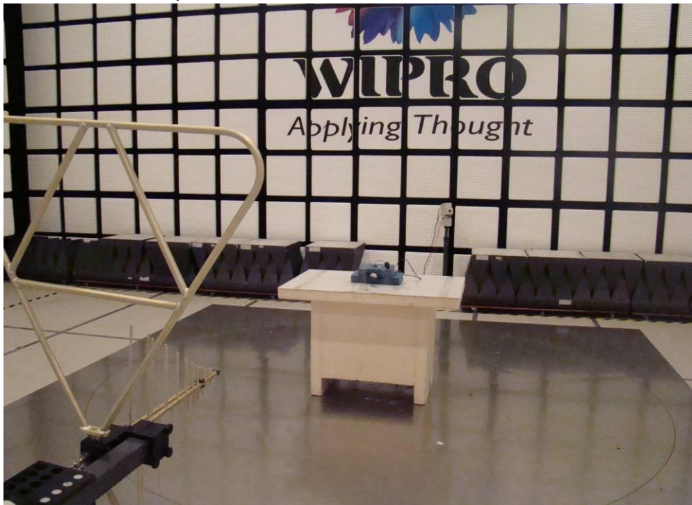
Radiated Test setup
