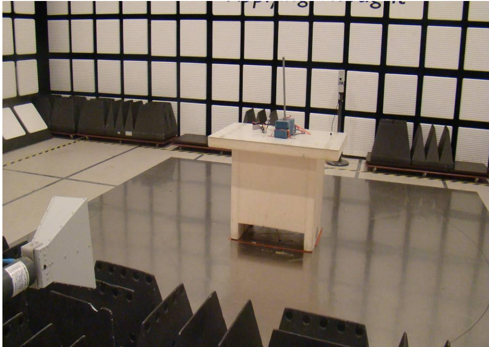
Radiated Test setup
