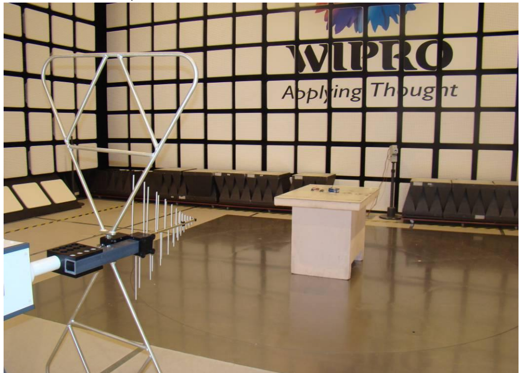
Radiated Test setup
