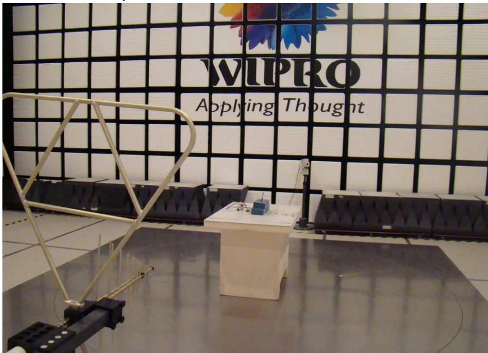
Radiated Test setup
