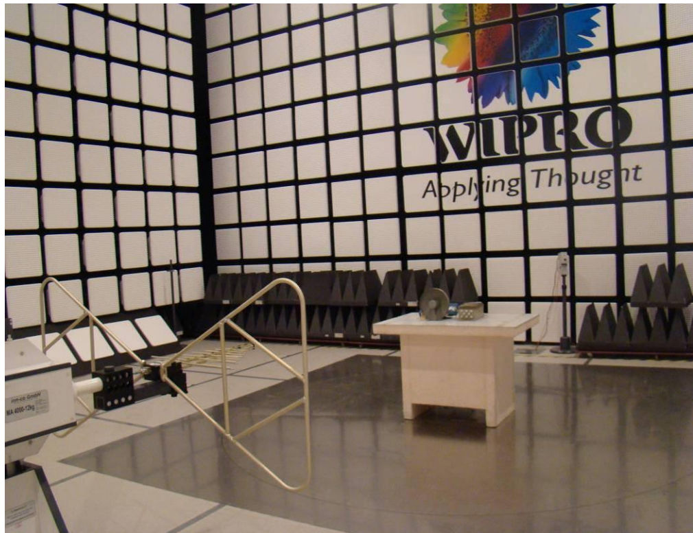
Radiated Test setup: Module inside host
