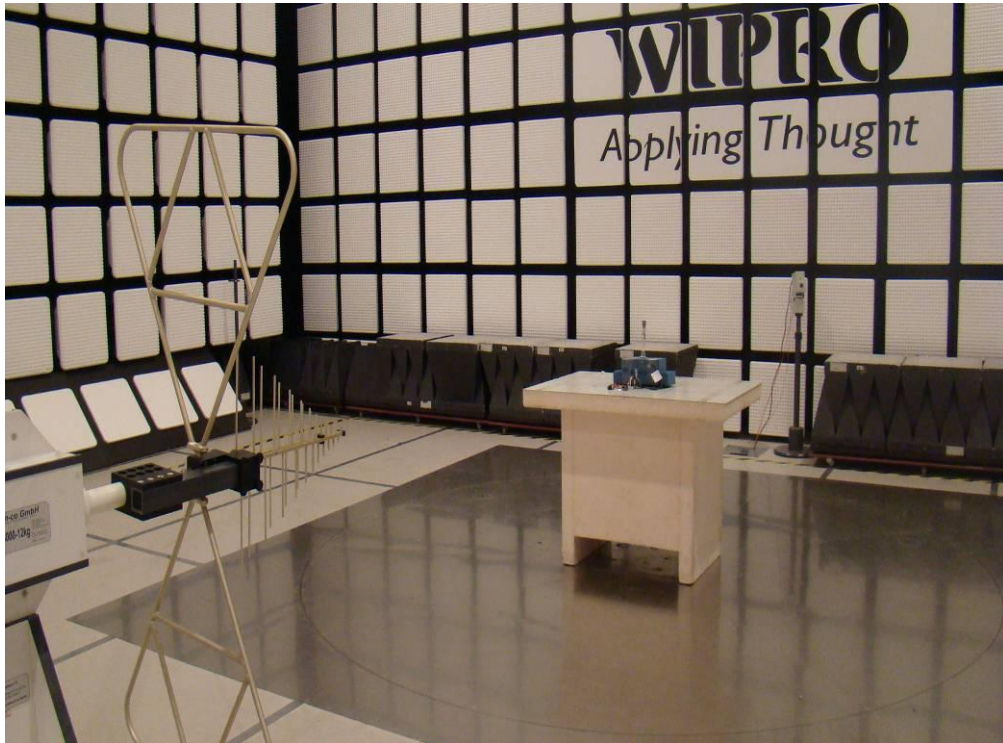
Radiated Test setup
