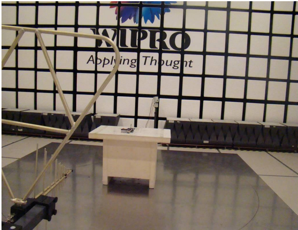
Radiated Test setup
