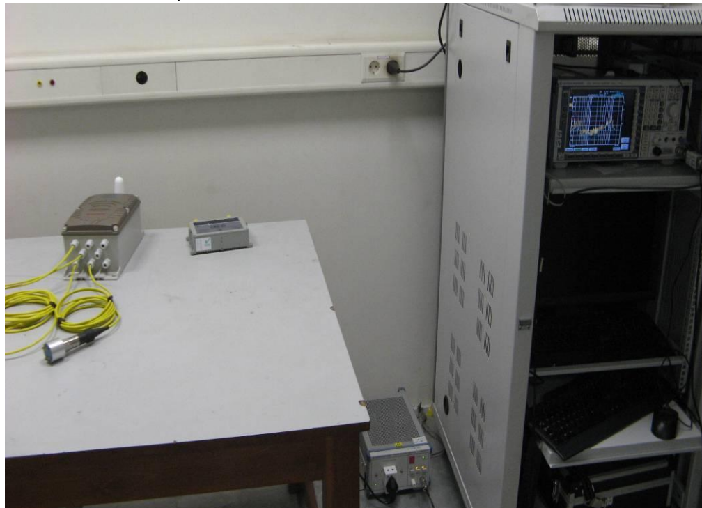
Test Setup: Conducted Emissions on Mains – with Module inside Host
