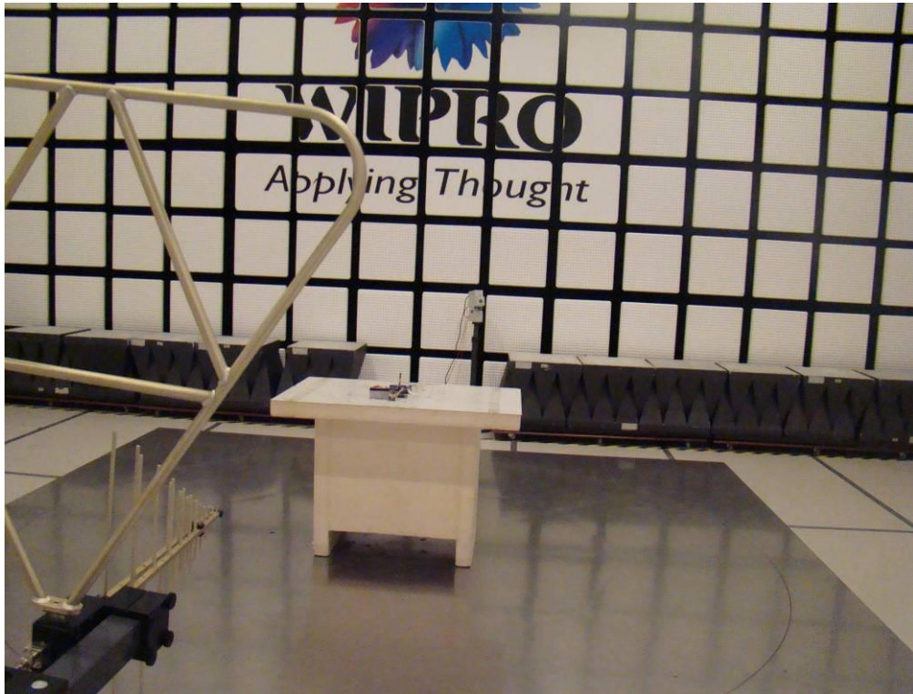
Radiated Test setup
