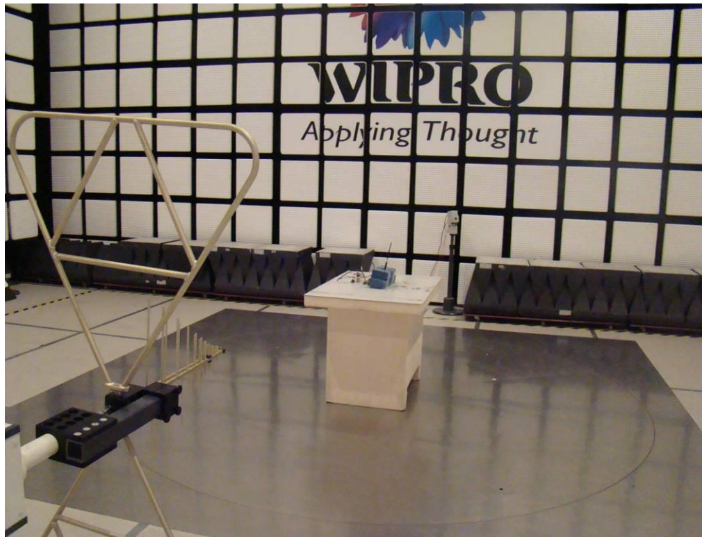
Radiated Test setup
