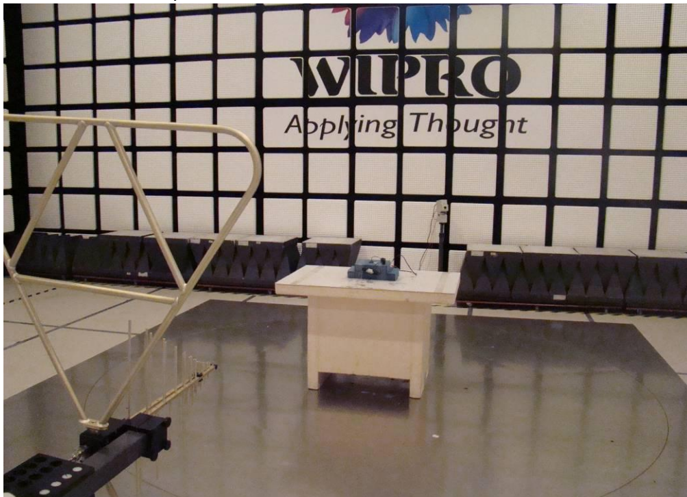
Radiated Test setup
