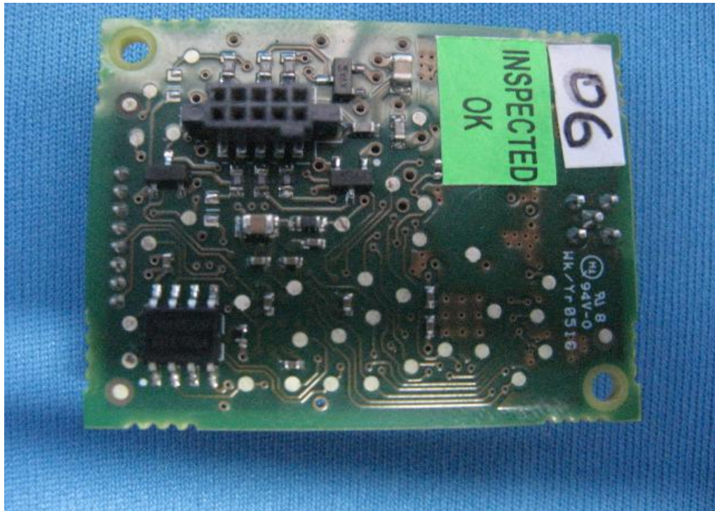
EUT Top Layer's Bottom View
