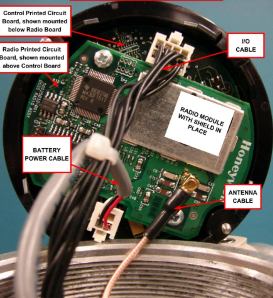
ELECTRONICS MODULE SHOWN REMOVED FROM
