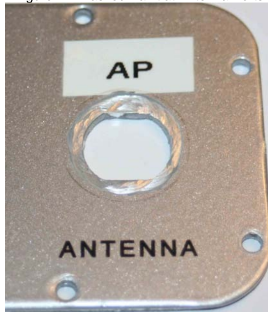
Figure 11: Masked Paint at Antenna Ports
