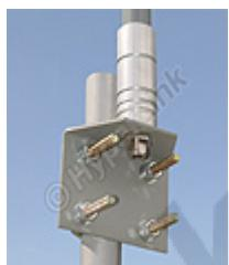
The HG5412U construction features a .96" diameter gray fiberglass radome for durability and aesthetics. It is designed for all weather operation. The integral N-Female type connector can be mounted through the wall of an equipment enclosure or to a mast up to 2.0" in diameter with the included mast mounting kit. The mast mounting kit consists of a heavy-duty steel bracket and a pair of U-bolts
