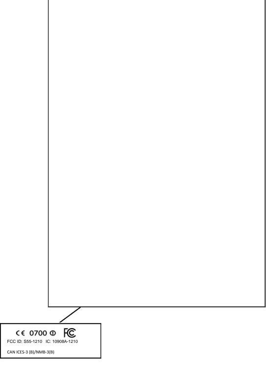
Location of this label – on the bottom back of the device
