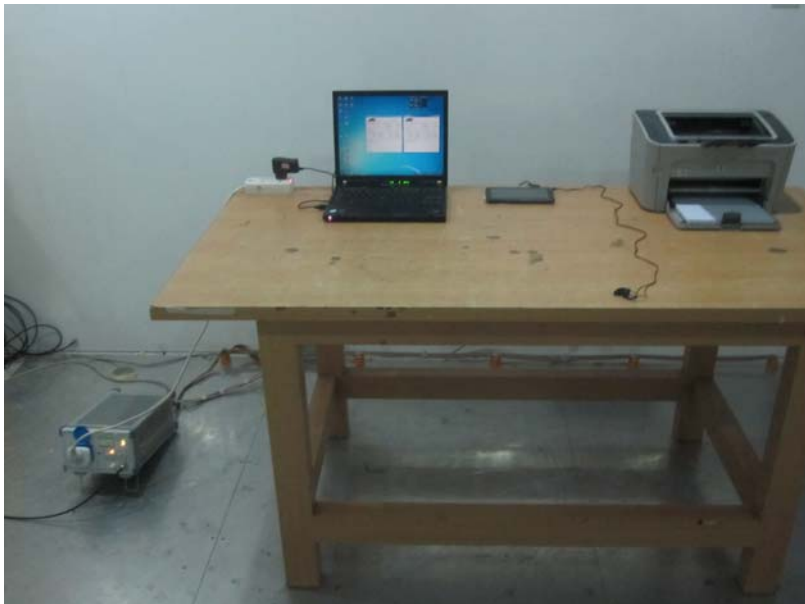
Photo of Setup for Conducted Emission
