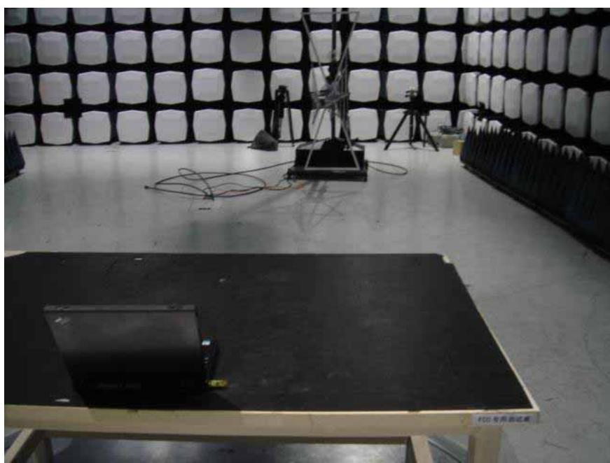
**2. Radiation Emission Test View For 1GHz-25GHz**
