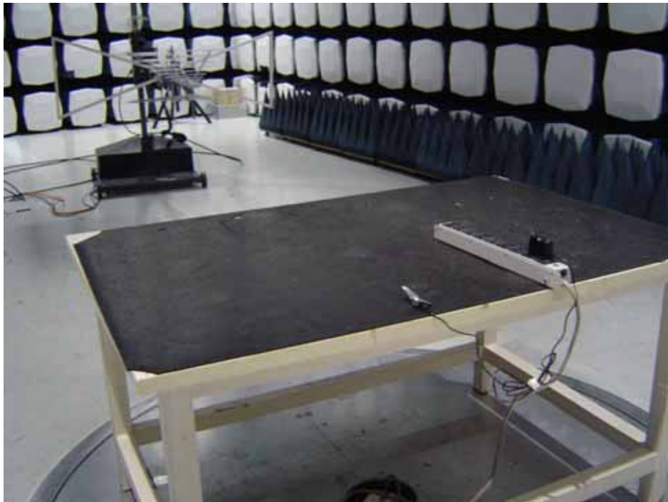
Radiation Emission Test View For 1GHz-25GHz
