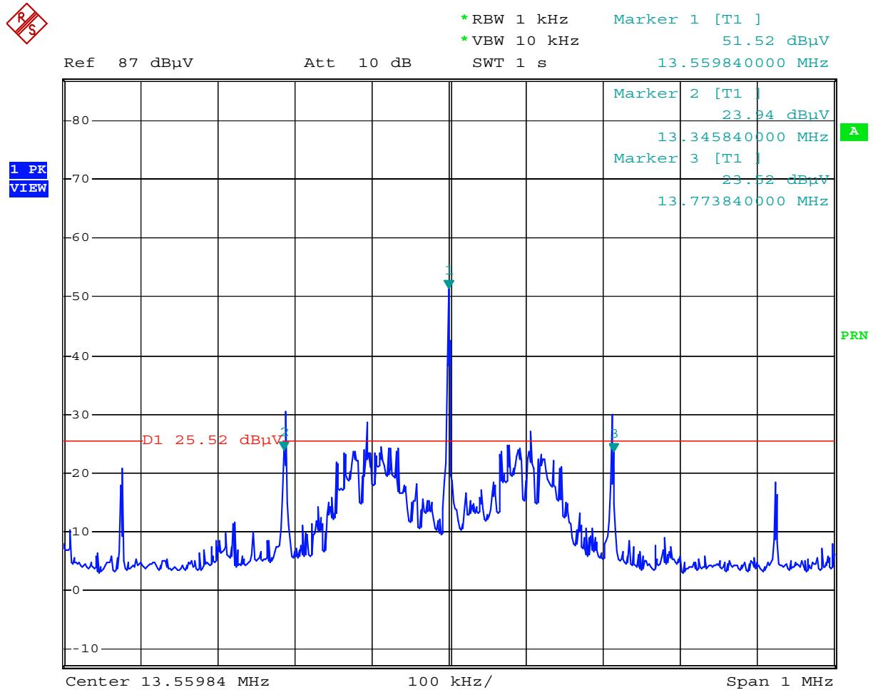
Occupied Bandwidth (-26 dB): **428 kHz**
