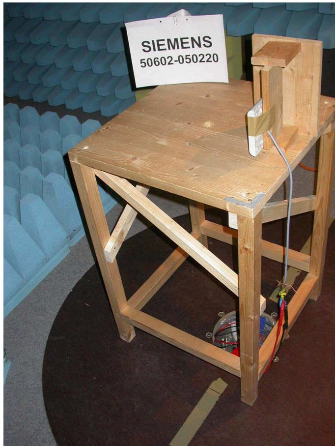
**Test setup for radiated emission measurement
