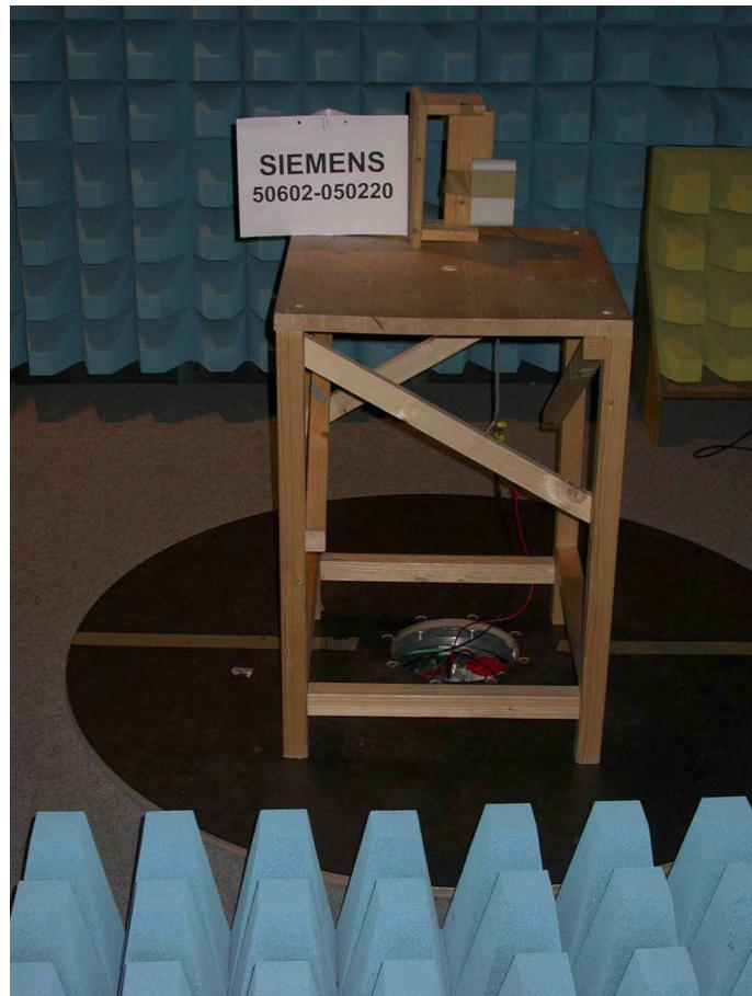
**Test setup for radiated emission measurement
