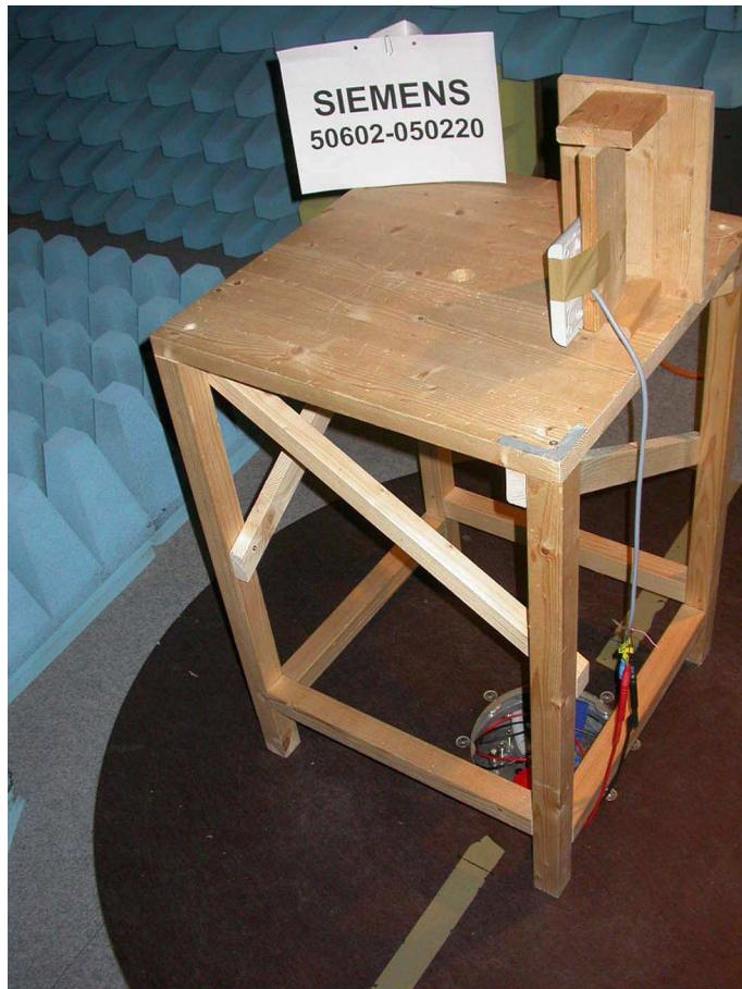
**Test setup for radiated emission measurement
