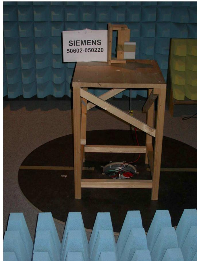
**Test setup for radiated emission measurement
