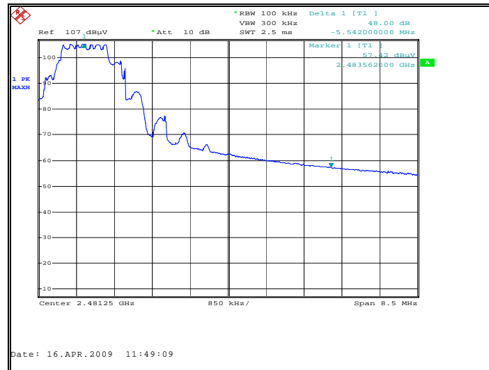
Figure 7.6.1.2-2: High Channel Band-edge Plot – Y-Position
