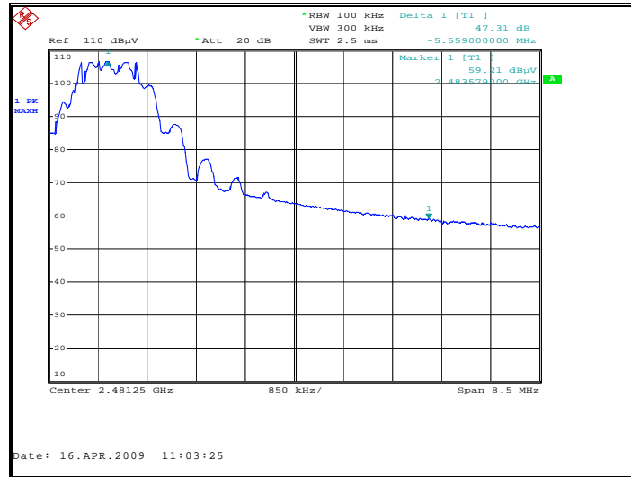
Figure 7.6.1.2-1: High Channel Band-edge plot – X-position
